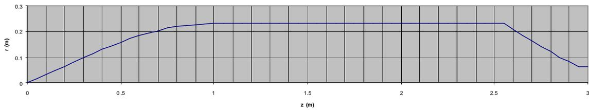
Figure C.7.2-1: The inner surface profile of the Phase1a beam dump
