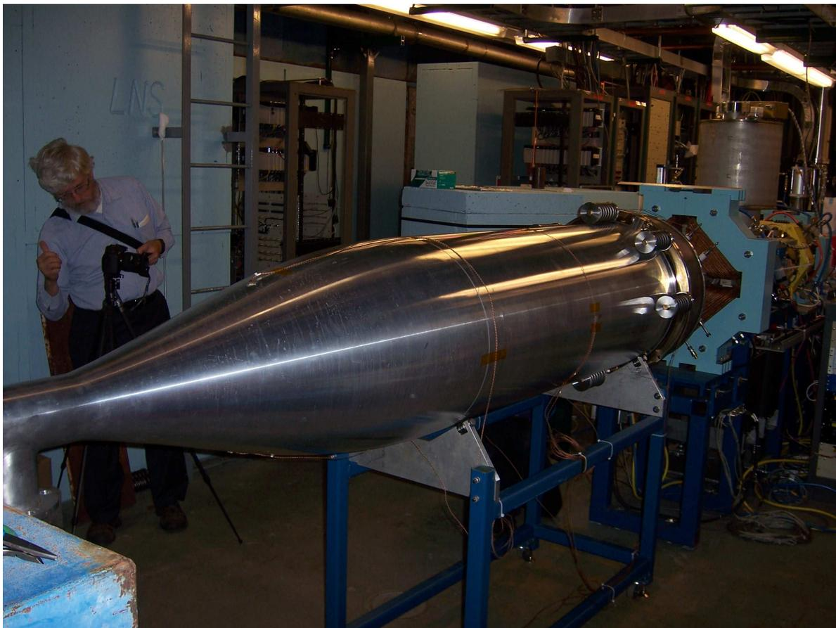
Figure C.7.2-2: The completed Phase1a beam dump before installation of its shielding.
