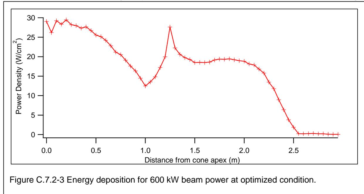
Figure C.7.2-3 Energy deposition for 600 kW beam power at optimized condition.
