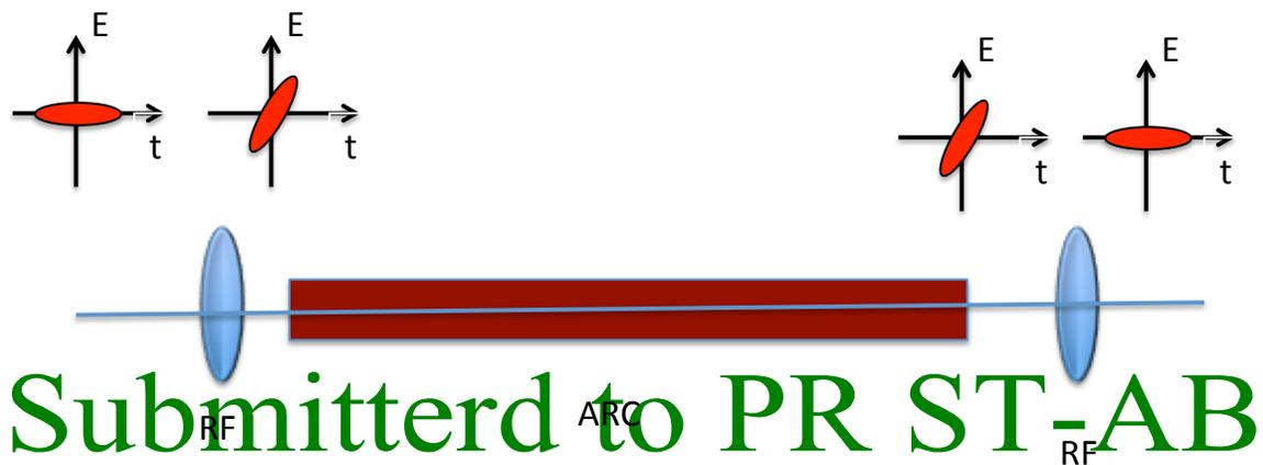
Figure 6. A sketch of a dedicated TBBU suppressor: One RF cavity gives an energy chirp to the electron beam at the entrance to the arc, and the other cavity removes the chirp.
