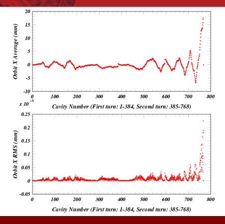
Each of the 384 cavities shows up twice in these plots, once for the accelerating pass and once for the decelerating pass.
