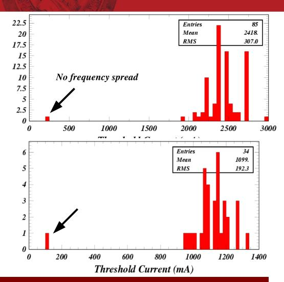
Offsetting the cavities horizontally with an rms value of 0.1 mm lowers the BBU instability threshold current from about 2400 mA to 1100 mA.
