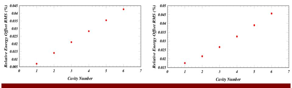
Second-order tracking through cavities induced 1.5e-4 relative energy offset in the 204 cavities upstream of the cryomodule with the 6 HOMs.
