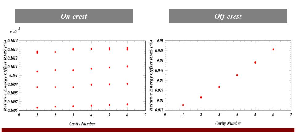
Energy spread increases by a factor of 3 from 0.016% to 0.045%.
