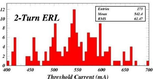
Modelled BBU instability thresholds for the case of polarized HOMs with 50 MHz HOM frequency splitting excited in each cavity of the full 1-turn Cornell ERL optics (upper plot) compared to the threshold currents calculated for the same case in the 2-turn ERL (lower plot).
