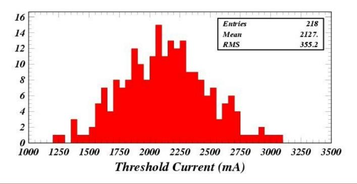
Modelled BBU instability thresholds for the case of a single higher-order mode excited in a single cavity of the fully coupled single-turn ERL optics in Ref. ERL-06-01 with polarized HOMs with 60 MHz frequency splitting and 10 MHz HOM frequency spread.
