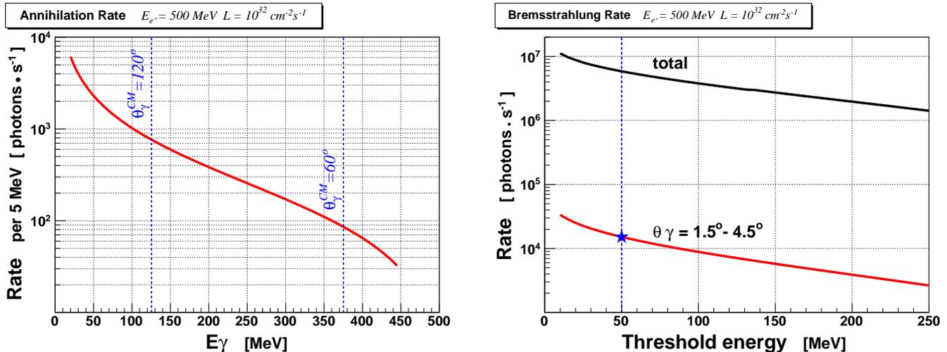
FIG. 4. Expected background photon rates at beam energy  $E_+ = 500$  MeV and luminosity  $L = 10^{32} \text{ cm}^{-2} \text{ s}^{-1}$ . Left panel: from positron-electron annihilation. Dotted vertical lines indicate the range covered in the proposed measurements. Right panel: from positron bremsstrahlung on hydrogen. At a 50 MeV threshold, the expected rate for the proposed detector configuration is  $1.5 \cdot 10^4 \text{ s}^{-1}$ .
