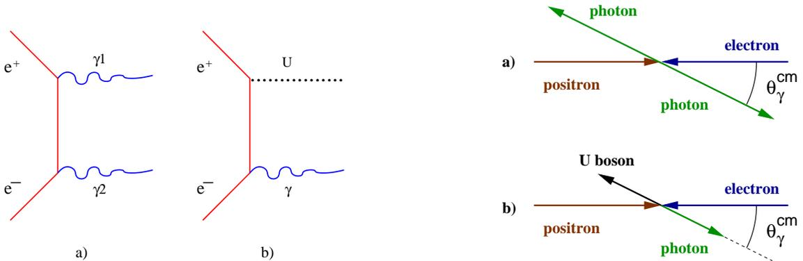
FIG. 2. The diagrams: a) two-photon annihilation, b) the U-boson- $\gamma$  production. The kinematics of  $e^+e^- \rightarrow \gamma + \gamma$  and  $e^+e^- \rightarrow U + \gamma$  reactions.
