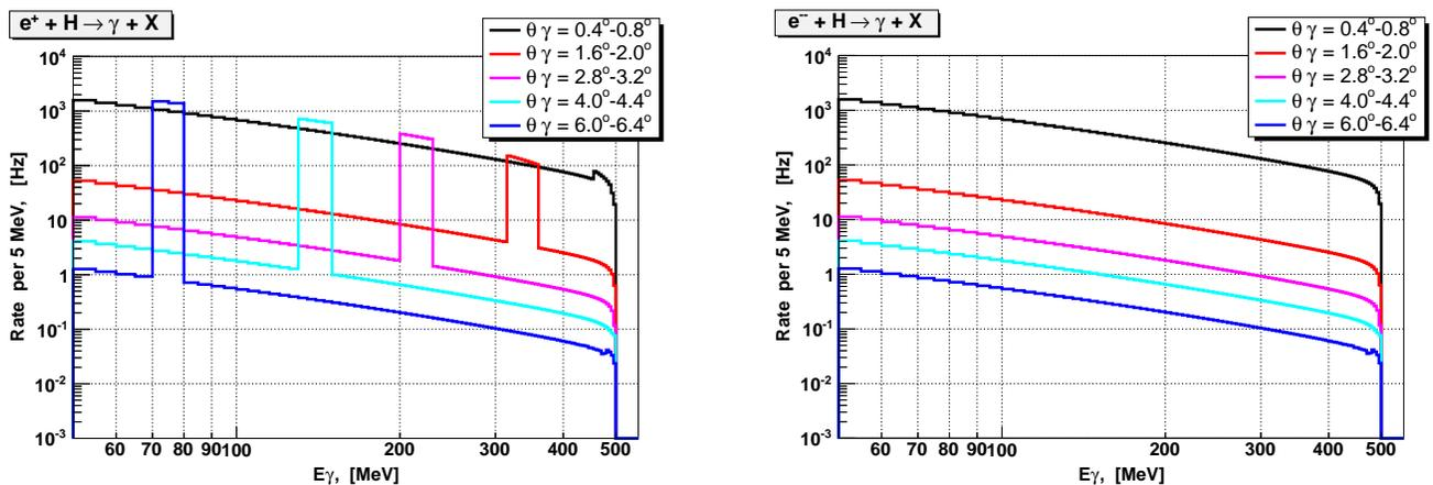
FIG. 7. The photon spectra in the case of a positron beam (left panel) and an electron beam (right panel) incident on an internal hydrogen target with a  $6.5 \cdot 10^{14}$  at/cm<sup>2</sup> thickness. Beam energy is 500 MeV and beam current is 25 mA in both cases. Bumps on the left panel, whose positions are moving with the scattering angle, are due to positron-electron annihilation process.
