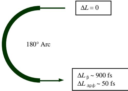
Figure 3: Conceptual 180°-bend arc and the estimated path length deviations. Note the 80°-bend does not necessarily consist of one dipole only.
