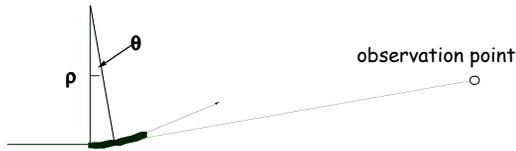
Figure 6: Geometry for the simulation of radiation. Distance between an observation point and a radiation point on an ideal orbit is 5 m.
