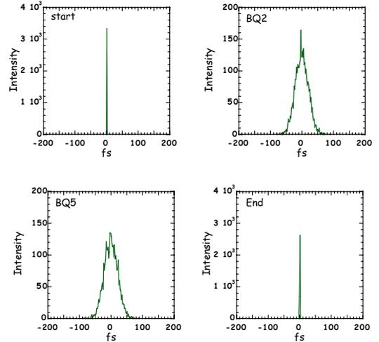
Figure 5: Tracking results for the path length deviation. Start (left-upper) and End (right-lower) mean the entrance and the exit of the 180° arc, respectively. BQ2 and BQ5 represent the middles of the 2<sup>nd</sup> bend and 5<sup>th</sup> bend in the 6<sup>th</sup>-unit-cell, respectively. The path length difference resulted from the betatron motion in the arc is almost cancelled out as one can see.
