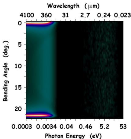
Figure 7: Calculated two dimensional spectrum of the SR from one of 6-unit-cell bending magnet. Coherent part can be seen at the left.
