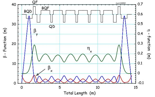
Figure 4: One of designed lattices for 180° arc. All bending magnets are combined function. Bending radiuses for the unit-cell bend and the dispersion suppressor are 3 m and 2 m, respectively.
