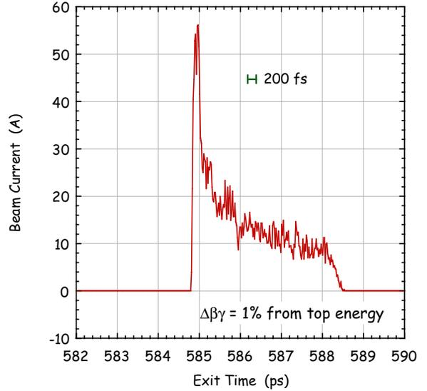
Figure 2: Example of simulated beam time spectrum from the ITC-Gun with 100 A/cm<sup>2</sup> cathode current. The spectrum is selected within a 1% energy width from a top energy electron.
