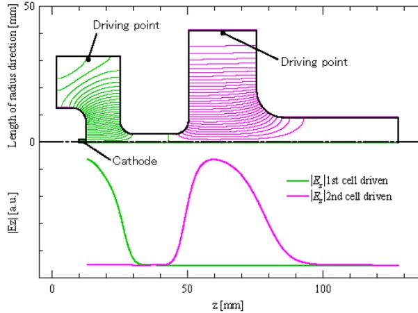
Figure 1: Calculated longitudinal electric fields excited in each cell. One can see the coupling between cells is almost negligible.
