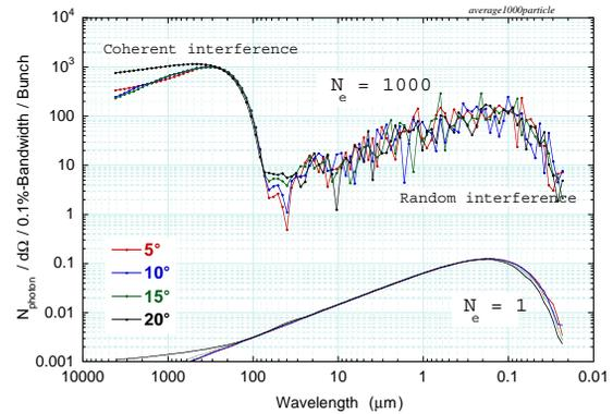
Figure 8: Calculated Spectra for different bending angles with one particle and 1000 particles. Intensity of coherent part is  $10^6$  times higher than that of one-particle is clearly seen. Because of the coherent edge radiation, the intensity at long wavelength is extraordinarily higher at the large angle.
