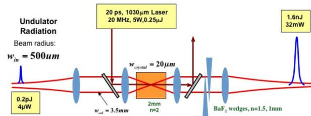
Figure 4: Layout of the optical amplifier.
