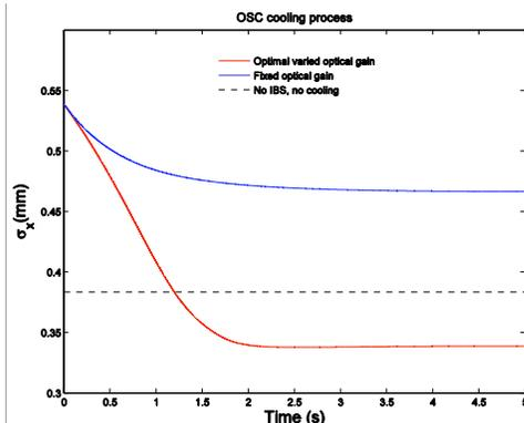
Figure 5: Calculated transverse size change due to OSC.
