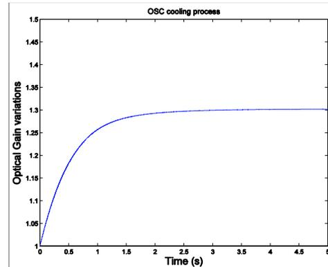
Figure 6: Optimal optical gain as beam cools
