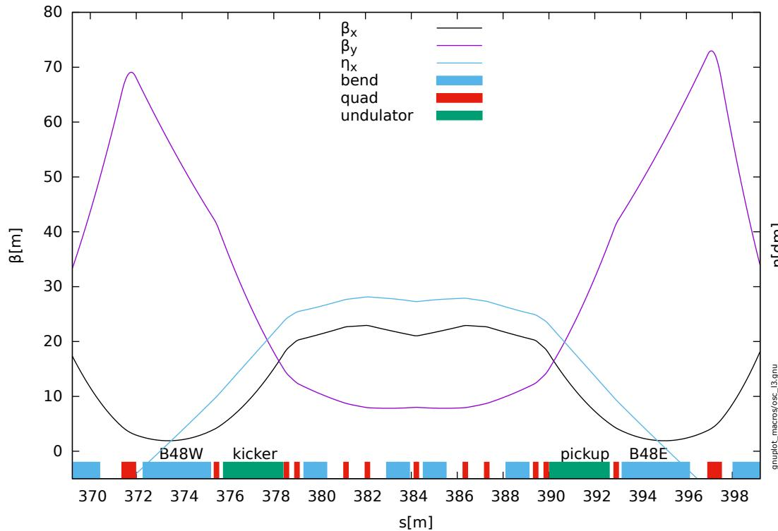
Optical stochastic cooling insert parameters
