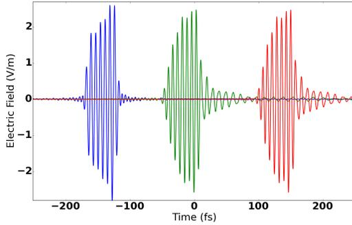
Figure 3: On-axis undulator radiation just upstream of the first lens (blue), its modification downstream passing through a 5-mm slab of BaF<sub>2</sub> using the implemented SRW model (green) and computed from Eq.4 (red). An artificial delay has been added to the pulses for clarity.
