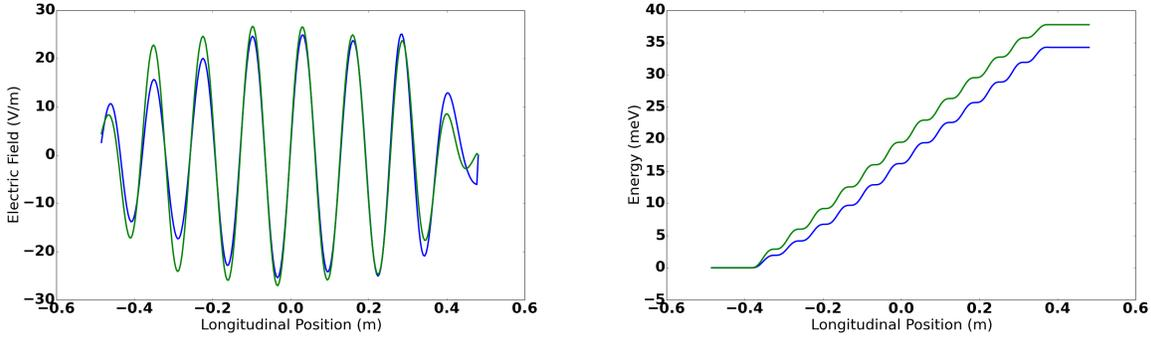
Figure 4: Left: Electric field experienced by an electron in the kicker undulator with (blue) and without (green) dispersion (green). Right: Energy transfer from the radiation field to the electron integrated over the kicker-undulator length for a phase corresponding to the maximum kick.
