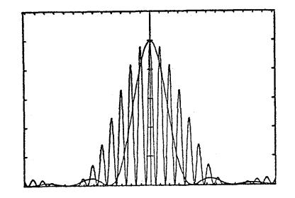
Figure 2 Curve of  $\lambda^4 \frac{dI}{d\lambda d\Omega}$  calculated for a single electron as a function of  $\frac{1}{\lambda}$  around the fundamental resonance wavelength in an optical klystron made of two 7 periods undulators. The dispersion corresponds to N<sub>d</sub> = 53 for the fast oscillating curve and N<sub>d</sub> = 0 for the smooth curve.
