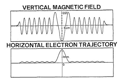
Figure 1 Vertical magnetic field calculated for the Orsay Optical Klystron (gap = 33.00 mm) and the corresponding horizontal electron trajectory at an energy of 240 MeV.
