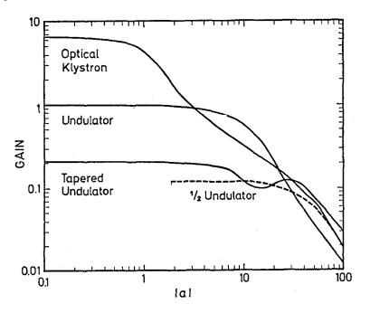
Figure 4 Maximum gain in relative units, as a function of |a| the generalized dimensionless laser amplitude for an optical klystron with D = 3, a regular undulator and a tapered undulator with  $\delta = 10 \pi$  (respectively), all three having the same total length
