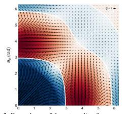
Figure 2: Dependence of the net cooling force on normalized betatron and synchrotron amplitudes in the linear approximation for  $k_0s_0=0$ . Vector field shows direction of the net cooling/heating.
