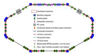
Figure 3: Schematic diagram of the Integrable Optics Test Accelerator ring at FNAL. The base configuration shown here is for the demonstration of nonlinear integrable optics; in OSC configuration, the lower straight is replaced with the insertion shown in Fig. 4.
