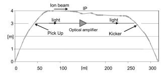
FIG. 3. Possible layout of a cooling system. The magnet-free area in the IP region is used for the pickup and kicker wigglers. (Focusing and bending magnets are shown on the plot with thickening of the lines. Vertical and horizontal axes show the scale of the transport line.)
