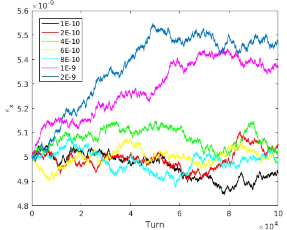
No cooling observed, probably due to incorrect model of incoherent kicks when having longitudinal structures (micro-bunching).
