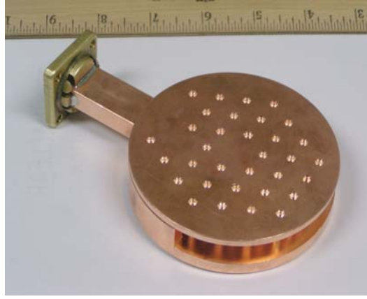
Figure 4-11: Brazed PBG resonator.
