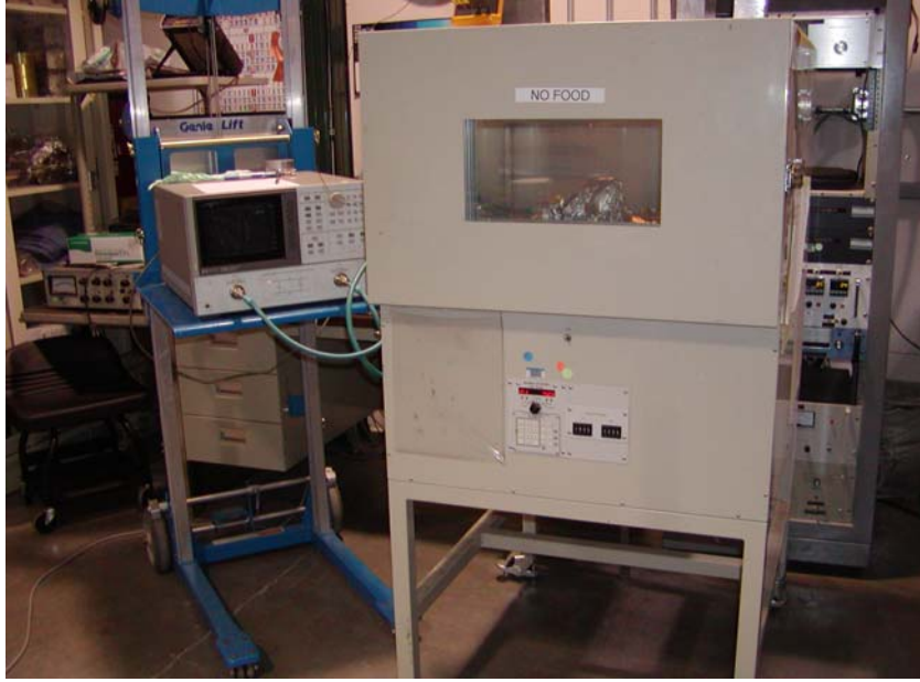
Figure 6-22: PBG structure inside the heating oven.
