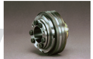
SKL Series 44-45 Major Feature: Single Point 360° Re-engagement and Sliding Bearing for Small Pulleys. Bore Range: 10 mm - 62 mm Torque Range: 2 Nm - 1500 Nm
