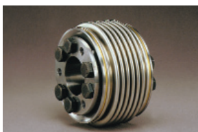
14-15 KSD Series Major Feature: High Clamping Forces, Maximum Misalignment and Short Length. Bore Range: 15 mm - 97 mm Torque Range: 20 Nm - 2500 Nm
