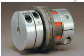
36-37 SEA Series Major Feature: Single Point 360° Re-engagement and Dampening Capabilities. Bore Range: 8 mm - 70 mm Torque Range: 2 Nm - 550 Nm
