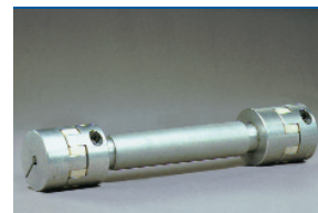
EKZ Series 22-23 Major Feature: All Aluminum Design, Lengths up to 2 Meters and Excellent Dampening Capabilities. Bore Range: 10 mm - 70 mm Torque Range: 20 Nm - 700 Nm
