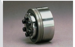
SKG Series 42-43 Major Feature: Single Point 360° Re-engagement and Integrated Bearing for Pulley Support. Bore Range: 12 mm - 62 mm Torque Range: 2 Nm - 1500 Nm
