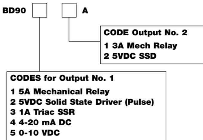
**Figure 1-2. CN9000A Series Replacement Output Board Numbering Information**
