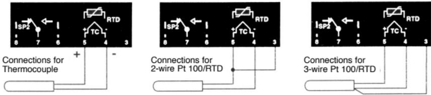
**Figure 2-4. Thermocouple and RTD Input Wiring**
