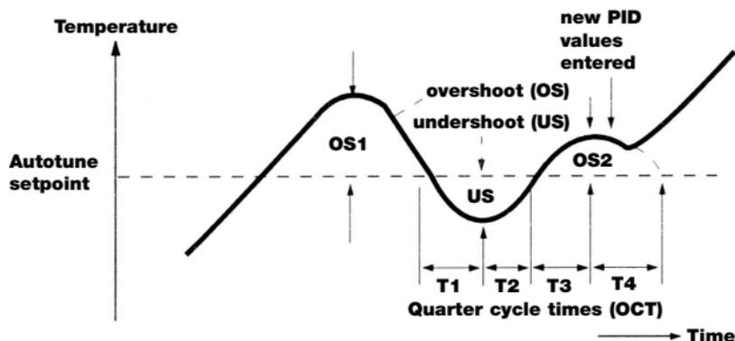
**Figure 4-3. Autotune Tuning Data (Functions .43-.49)**
