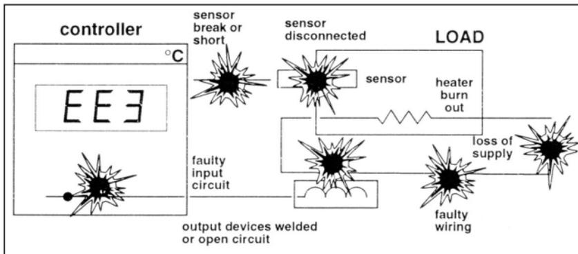
**Figure 4-1. Typical faults detected by LBA**
