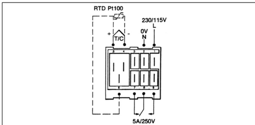
**Figure 2-7. Wiring of single output controller CN9110A, CN9210A**
