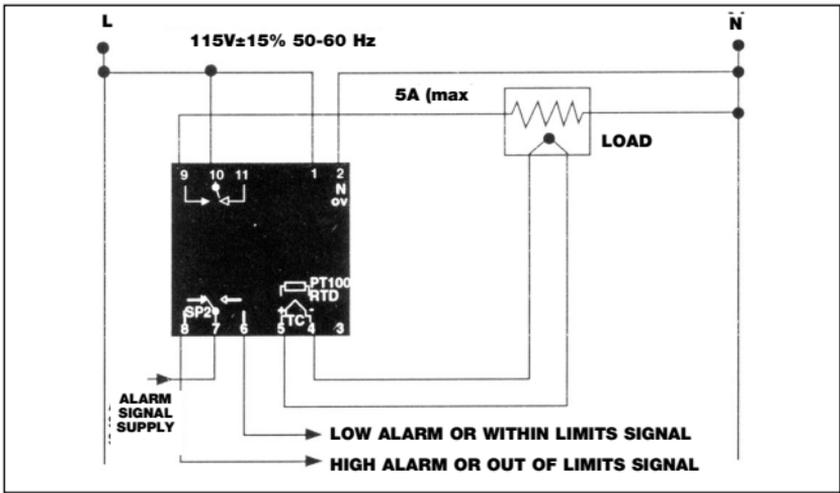
**Figure 2-5. Wiring Heater with Alarms (Two Mechanical Relays-Model CN9111A)**
