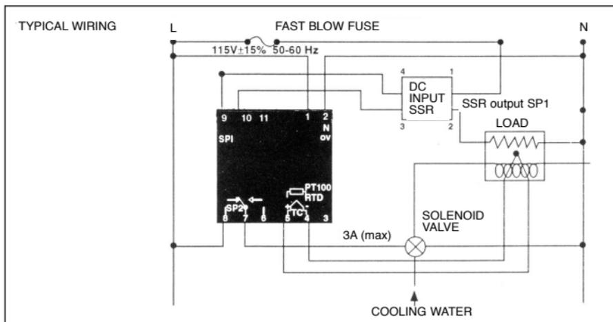
**Figure 2-6. Heating and Cooling CN9121A [One DC Solid State Relay Driver for Heating (SP1), 3A Mechanical Relay for Cooling (SP2)]**
