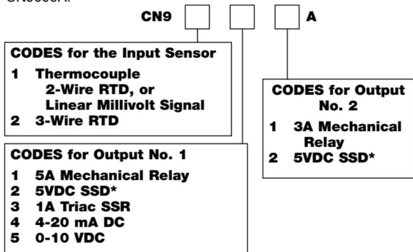
\*SSD output is a Solid State Driver (5 Volt DC Pulse) designed to be used with a DC controlled solid state relay such as OMEGA's model number SSR240DC45 relay.
