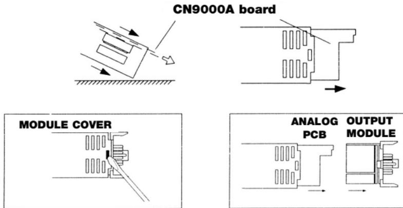
**Figure 7.1. Removing the Main PC Board**
