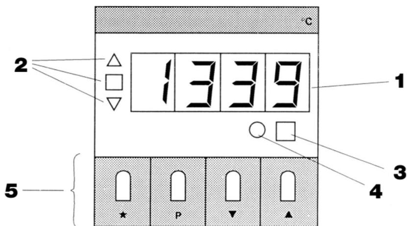
**Figure 3-1. CN9000A Front Panel-Controls and Indicators**
