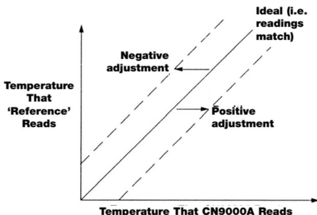
**Figure 6-1. Sensor Error Graph**
