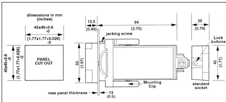
*\*To unplug socket, press in lock buttons and pull apart*
