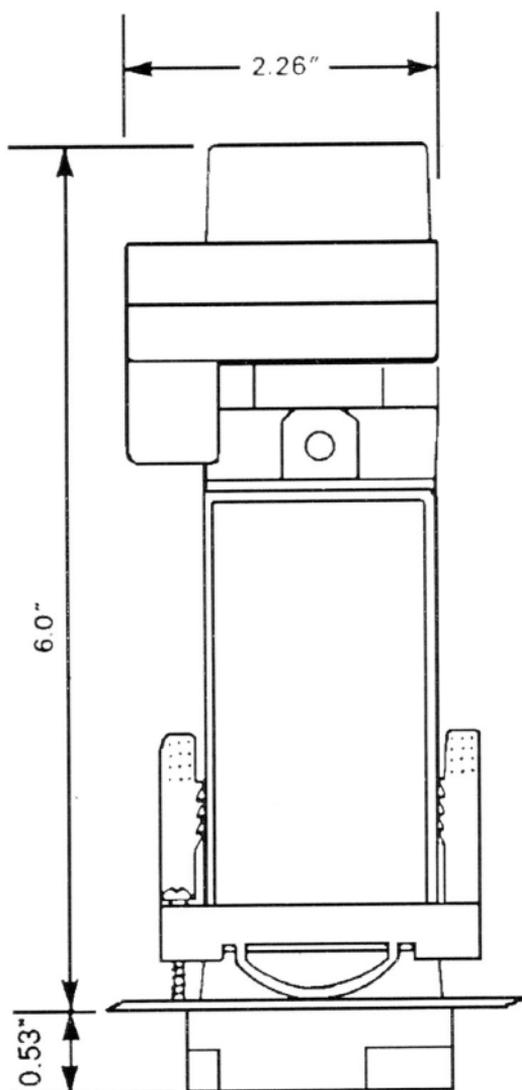
**Figure 8-1. Dimensions with the Power Socket**
