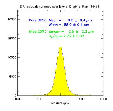
Residuals: time-measured hit position are compared to the fitted position.Parameterized as double gaussian with fixed 80% fraction in narrow component.
