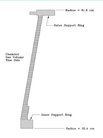
The outer section supports 31 anode layers and associated field wire layers. Layers are grouped in 8 stereo super-layers with equal number of cells per layer and half-cell-stagger.
