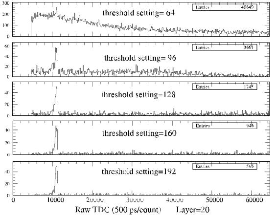
Threshold is set at 0.8  $\mu$ A. with a characteristic time of 8 ns (amplifier rise time), and gas gain ~  $10^5$ , threshold is 0.4 primary ions.
