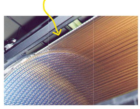
Segmented cathode forms the outer field cage for the outer (47<sup>th</sup>) layer.
