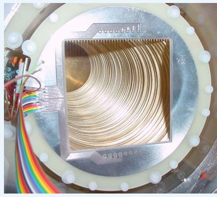
Positive ions are created in the amplification and drift back into the field cage.
