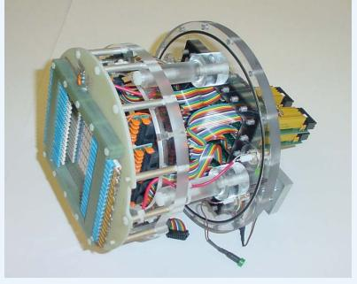
The readout module including the amplification device mounted on pad board
