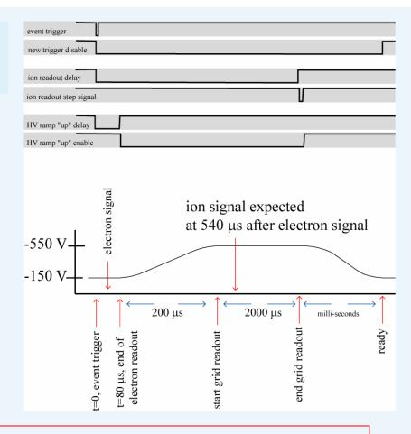
Require small ion drift time to reduce diffusion. (Expect ~7 µs diffusion at 540 µs drift.)
