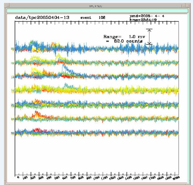
Note the 1 mv scale. Gas amplification is about 100
