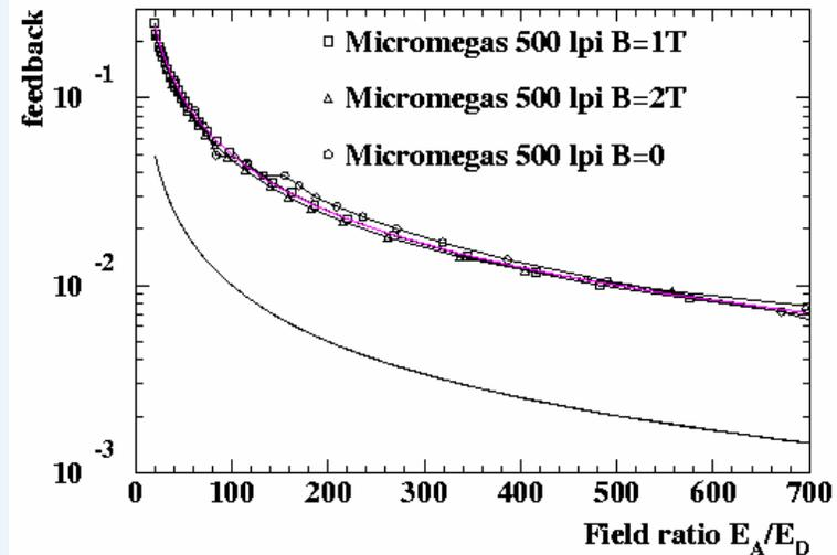
Ion feedback with Micromegas, P10
