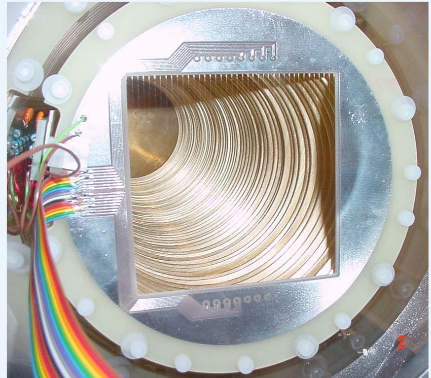
Positive ions are created in the amplification and drift back into the field cage.
