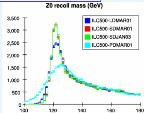
measure the mass recoiling against  $l^+ l^-$  in  $(e^+ e^- \rightarrow HZ, Z \rightarrow l^+ l^-)$
