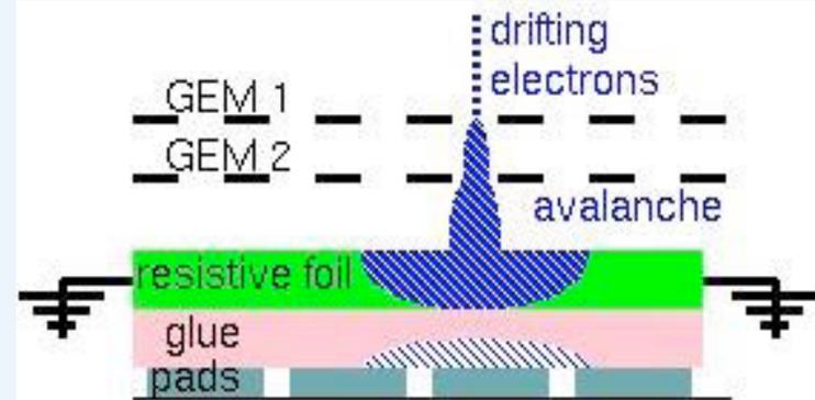
Charge dispersion with resistive anode
