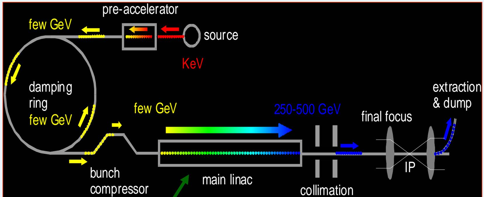
Superconducting RF Main Linac
