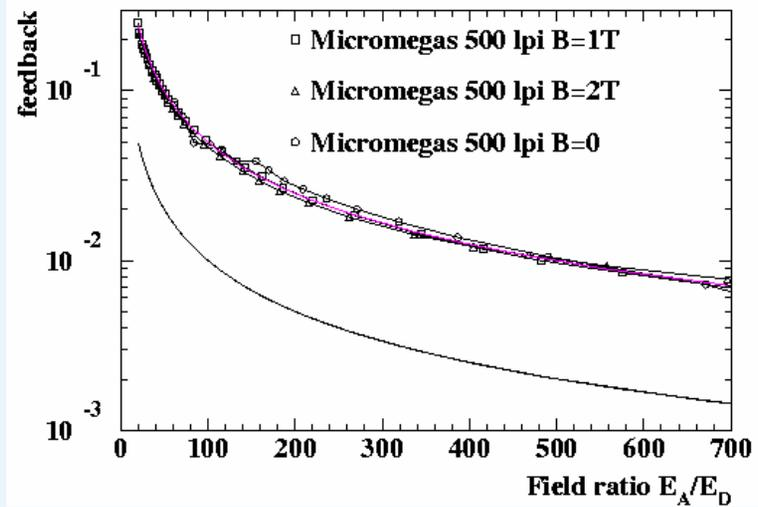
Ion feedback with Micromegas, P10
