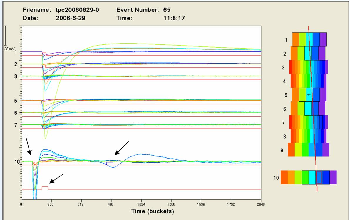
Pulse observed on field cage termination, is this ion feedback?
