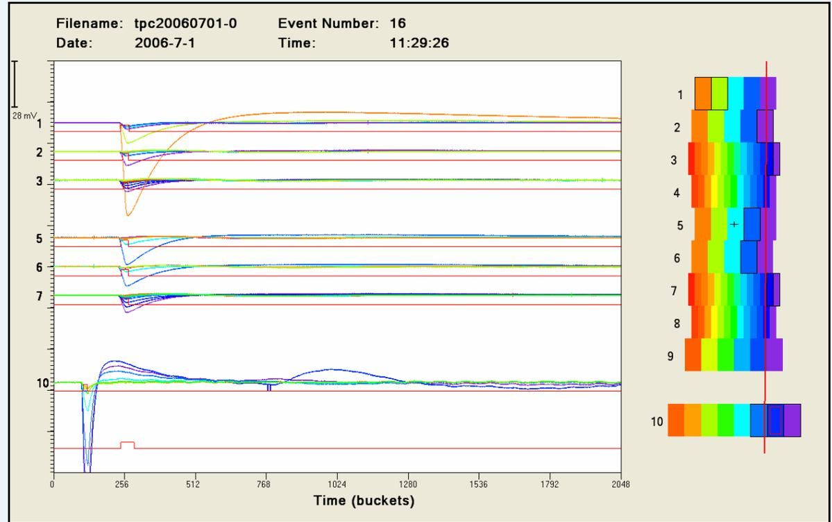
Pulse still observed on field cage termination; decreased signal to noise ratio makes pattern-recognition difficult
