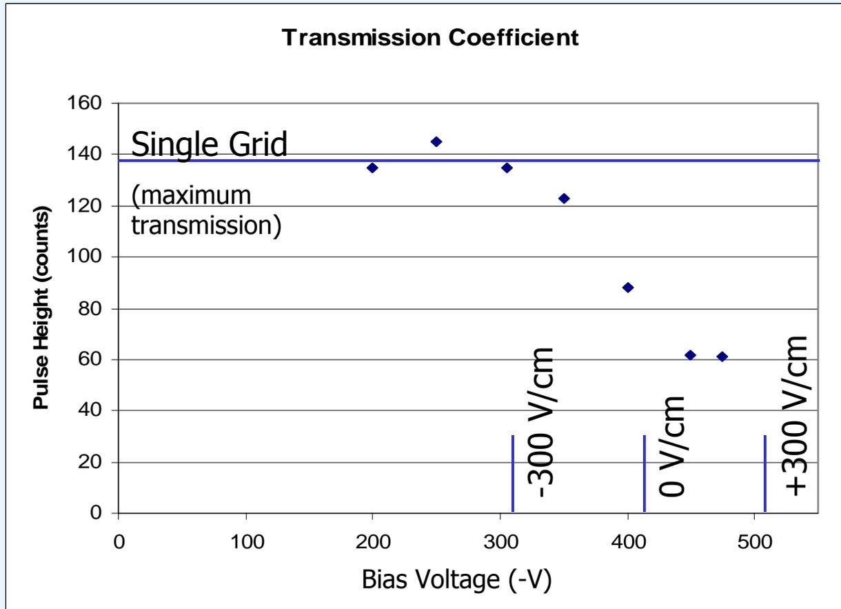
Transmission coefficient of electrons through double field cage termination wires using Micromegas
