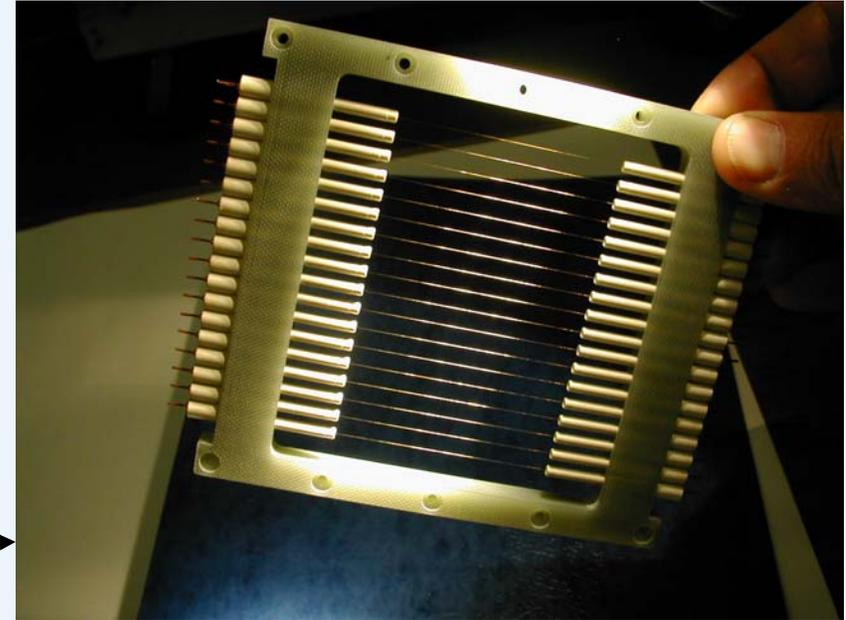
Wire amplifier produces large feedback signal this is why it is unsuitable for use in the ILC
