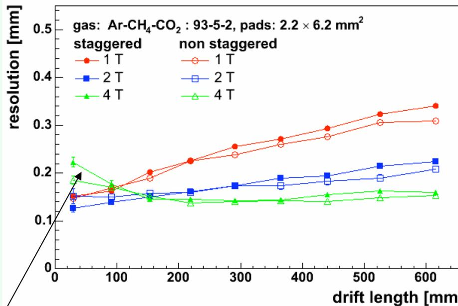
Rise indicates pad size is too large for signal width at 4 Tesla
