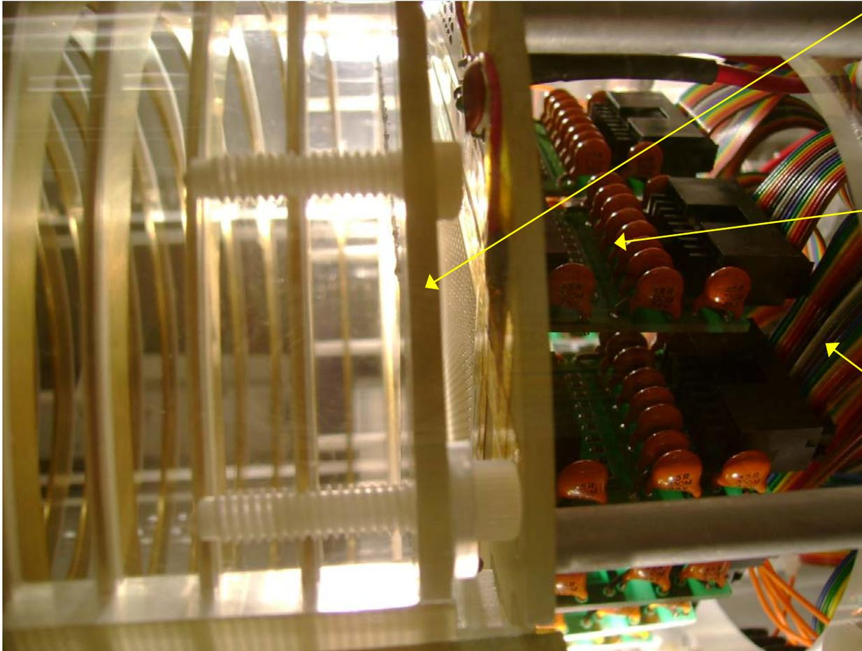
The Micromegas is located 0.78 cm from the field cage termination.
