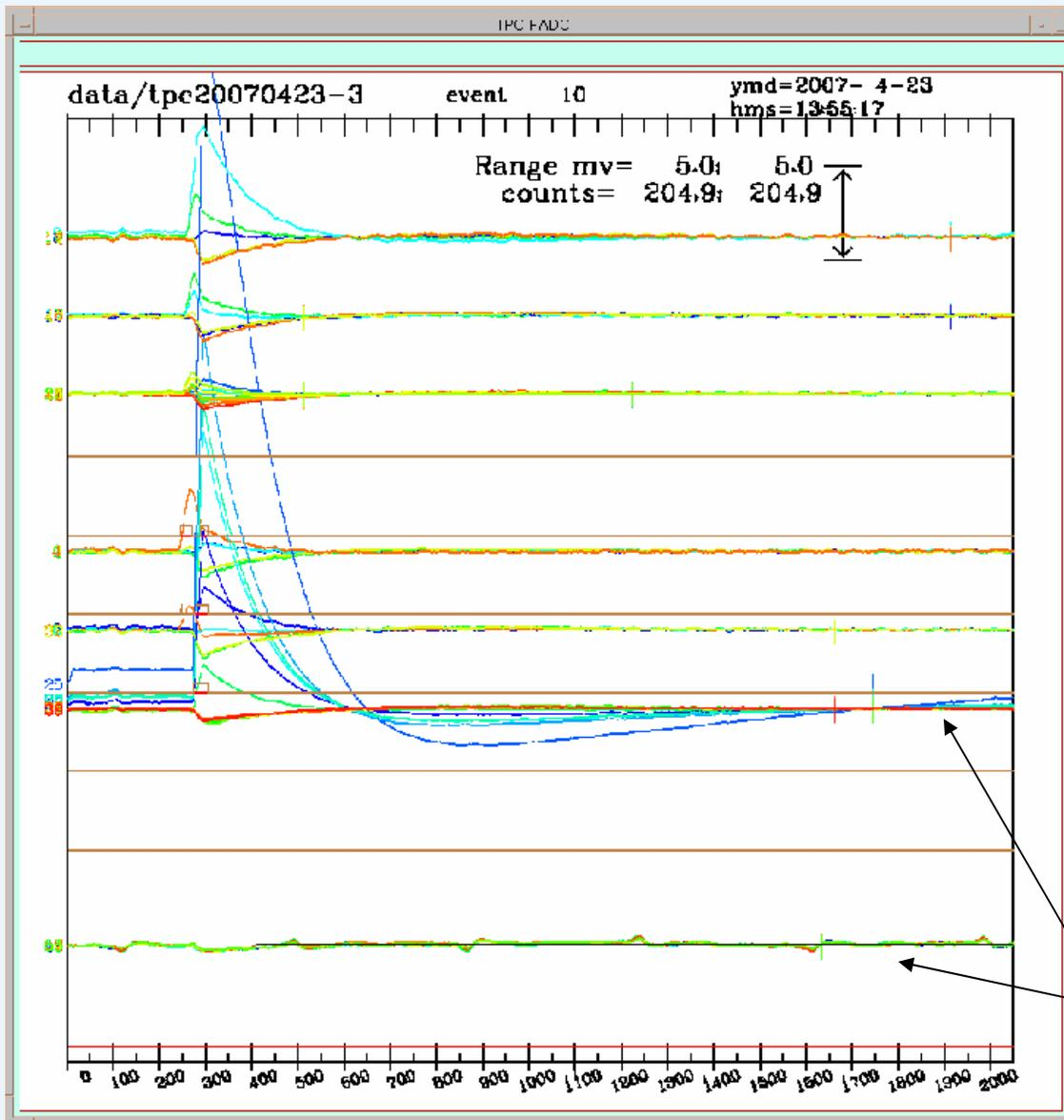
The "opposite signal" is observed in both the Bulk Micromegas and the Purdue-3M Micromegas.
