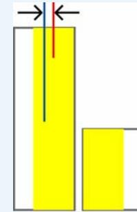
Here, the containment width of the pad distribution function is small; any sharing indicates that the charge center of each pad is not the geometric center. Thus, there is a shift of the effective pad center.
