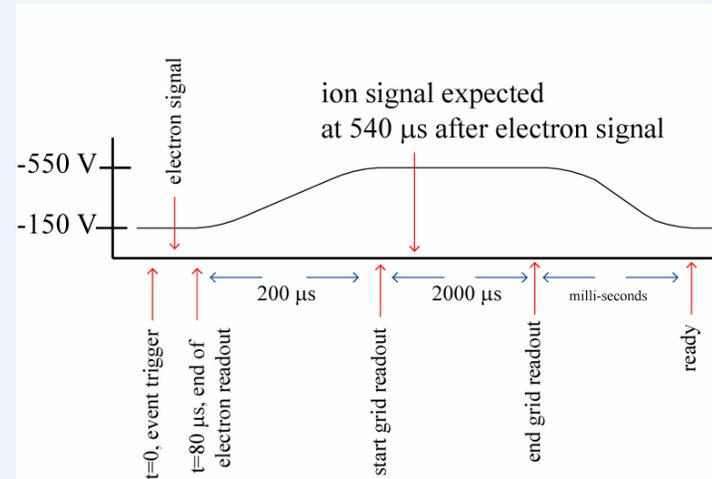
More sensitive measurements will require a pulsed bias on the field cage termination to provide full electron transmission and full ion collection.
