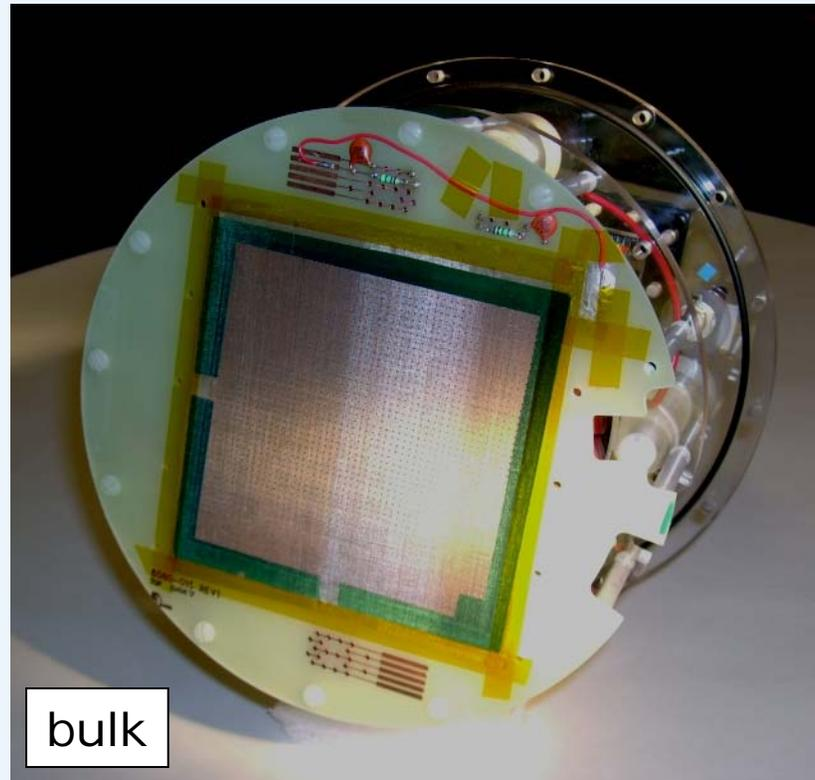
The “bulk Micromegas”, was prepared on one of our pad boards by Paul Colas’ group. Measurements with the Purdue-3M Micromegas were shown at Vancouver 2006.
