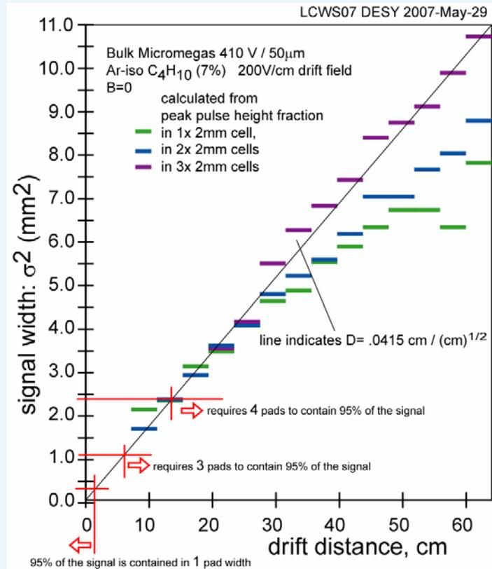
The charge width is determined from the fraction of the total charge in 1, 2 or 3 pads, shown above, assuming a gaussian charge distribution.
