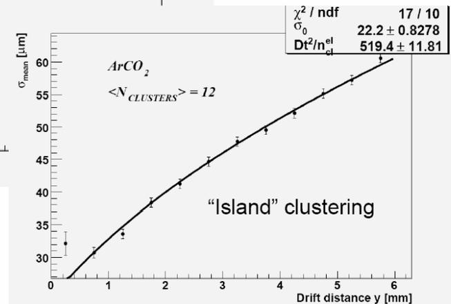
Two clustering methods were presented, with point resolution measurements.
