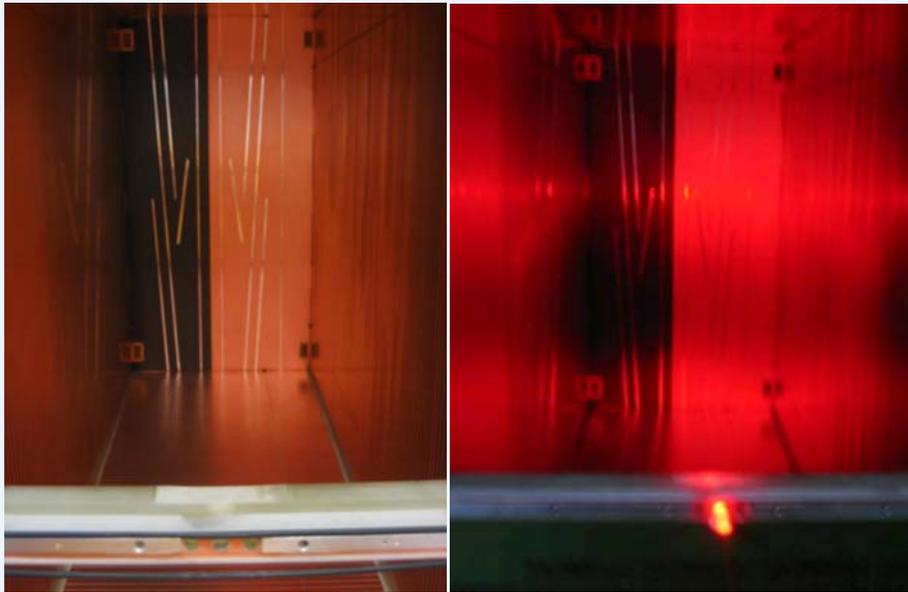
To produce photoelectrons for distortion measurements, place on the central cathode a pattern of metal with a lower work-function.
