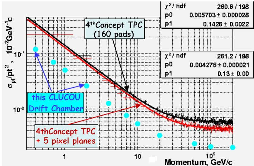
*The Reduced scattering and point resolution are expected to provide improved momentum resolution.*
