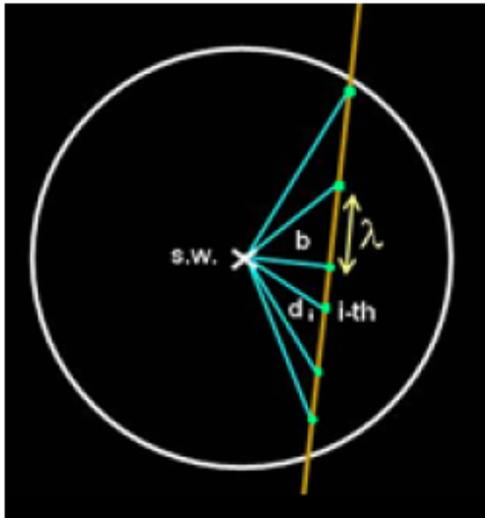
Sampling the drift chamber signal provides more information than the threshold-crossing time.
