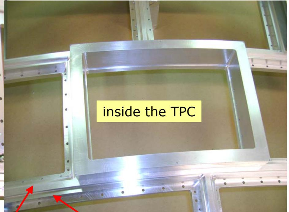
The stiffening rib could be made of fiber.
