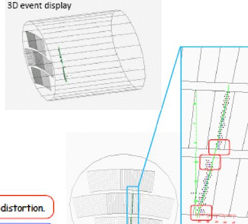
Metal posts facing drift volume produce local distortion.
