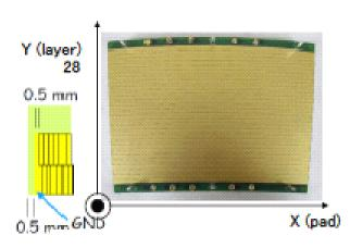
28 pad rows 192 pads at outer 176 pads at inner (1.15-1.25)mm W 5.26mm H
