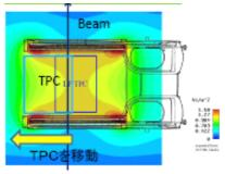
Displacing TPC in magnet for drift distnce dependence introduce different B for each drift as moving stage was not available
