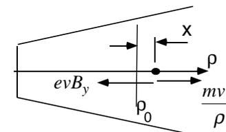
For radial stability, the centrifugal force must be less than the Lorentz force for  $x > 0$ :
