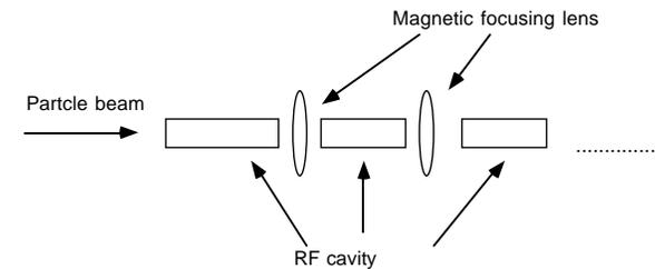
Lenses are required for transverse stability (the RF cavities are
