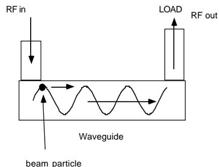
Typically operated in a TM mode: longitudinal electric field provides the acceleration. Beam is bunched, rides at crest of wave
