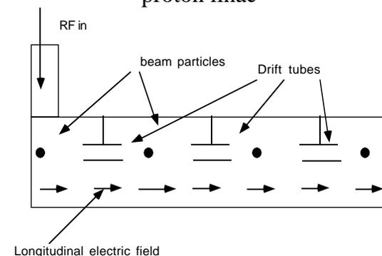
Beam is shielded from the fields when at the wrong phase by using hollow “drift tubes”
