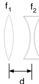
$\frac{1}{f} = \frac{1}{f_1} + \frac{1}{f_2} - \frac{d}{f_1 f_2}$  is positive for a large range of focal lengths and  $d \Rightarrow$  net focusing both radially and vertically
