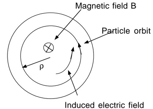
The orbit radius  $\rho$  is fixed. The accelerating electric field is provided by the changing magnetic flux within the orbit. The required flux change is  $\Delta\phi = 2\pi\rho^2 B_{\text{max}}$ . Energies up to 300 MeV have been obtained.
