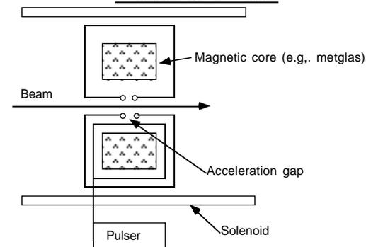
The beam forms the secondary circuit of a high-current pulse transformer
