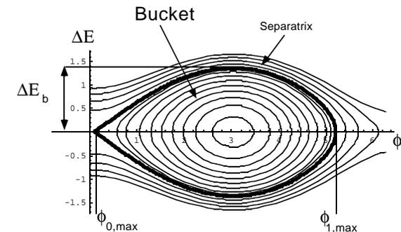
There are  $h$  such buckets around the machine, and there may be  $h$  synchronous particles at the center of each one. Thus the machine can contain at most  $h$  bunches.
