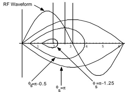
The rf bucket corresponding to  $\phi_s = \pi$ , for which there is no acceleration, is called a *stationary bucket*.
