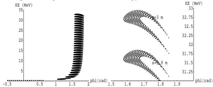
The output phase space has a full energy spread of about 1 MeV, and a full phase spread of about  $15^\circ$  (14 ps).
