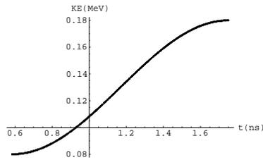
Longitudinal phase space just after the 214 MHz prebuncher
