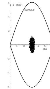
The rf voltage is adiabatically reduced to a small value  $V_{min}$ , over many synchrotron oscillation periods. The bunch remains matched to the bucket; the energy spread goes down like  $V^{0.25}$ , and the time spread (bunch length) goes up like  $V^{-0.25}$ . The product must remain the same by Liouville's theorem.
