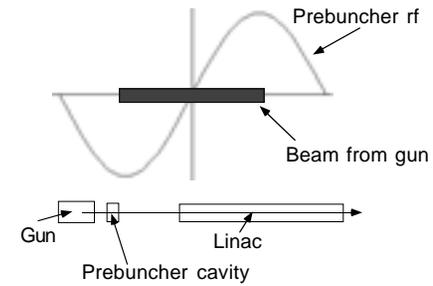
The beam from the gun is injected into the prebuncher cavity so that the early particles are decelerated, and the late ones accelerated.
