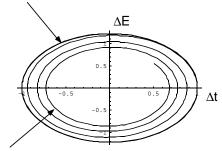
Damped trajectory with radiation power  $P \propto \gamma^2$
