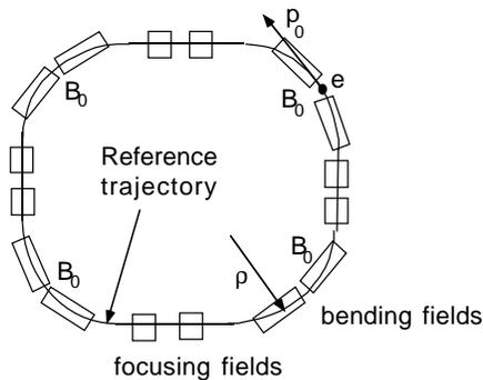
The “reference trajectory”  $\vec{r}_0(t)$  is the trajectory of a “reference particle” of momentum  $\vec{p}_0$  that passes through the center of symmetry of all the *idealized* magnetic guide fields. The reference trajectory is an *idealization*.
