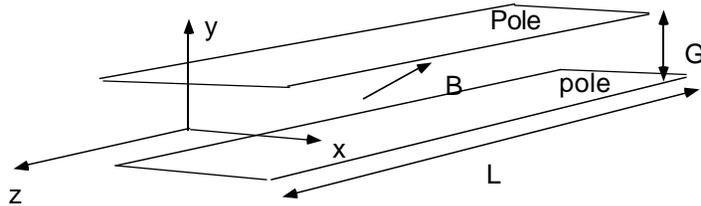
The *idealized fields* extend only over the length L (“effective length”) and are independent of z and transverse to the beam. Idealized fields ignore the fringe fields. (Note that this is does not
