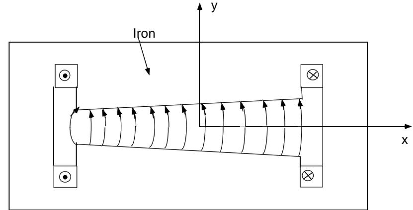
Gradient magnet (for combined function machines): provides both a bending field and a gradient (due to changing gap dimension).
