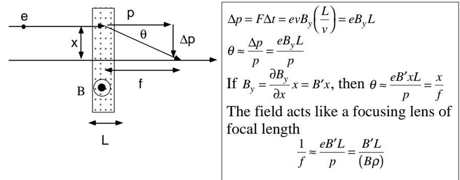
This linear dependence of field on position can be generated by a quadrupole magnet
