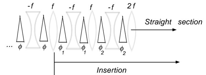
The insertion starts with two regular-strength FODO cells, in which the dipoles are operated at different bend angles,  $\phi_1$  and  $\phi_2$ , than the dipoles in the rest of the lattice (which have a bend angle  $\phi$ ). These cells are followed by a straight section, in which the dispersion will be zero. The insertion is symmetric about the center of the straight section.
