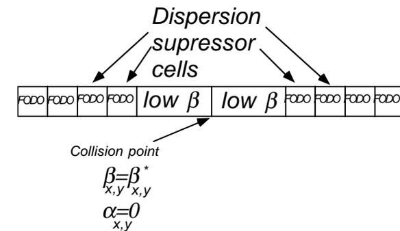
Two symmetric insertions are used, to match from the FODO lattice to the collision point. Dispersion suppression is also required.
