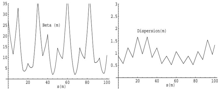
This produces major perturbations to the lattice functions (beta more than doubles) and is highly undesirable. The insertion needs to be *matched*. We’ll discuss several simple types of matched insertions.
