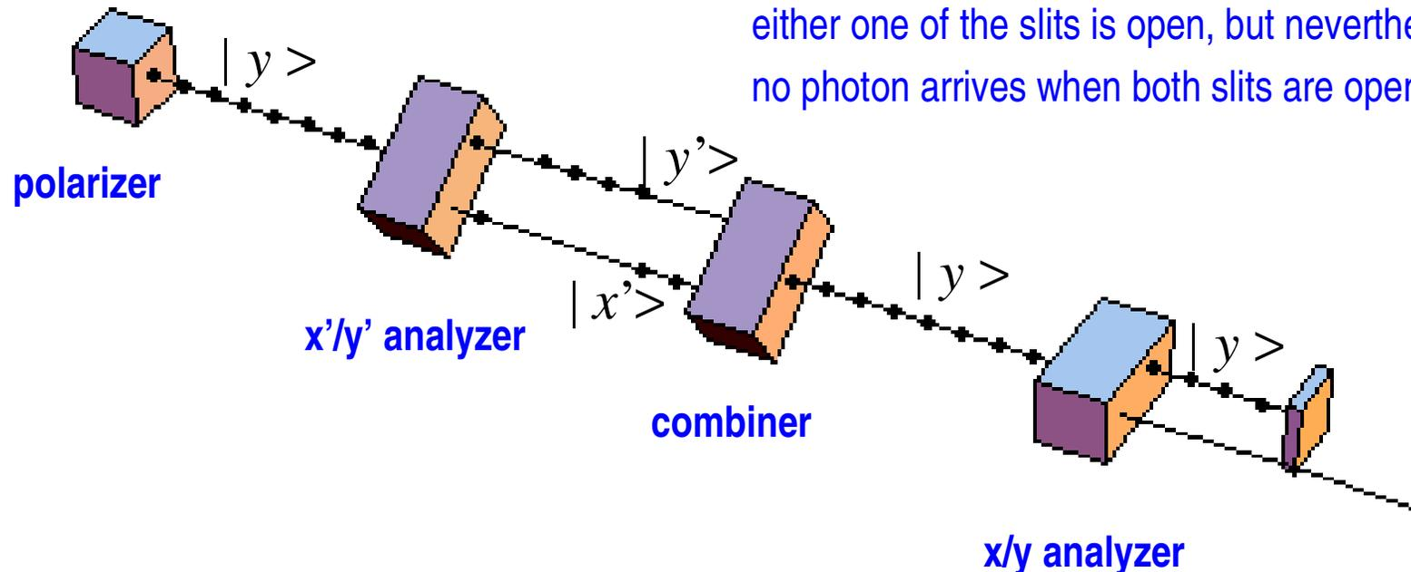
The output **intensity** of a light wave corresponds to the number of photons and therefore to the **probability** that a photon is found in the output channel. To have photon probabilities correspond to wave intensities, one introduces a **state vector** that describes photons and **can interfere** like the field vector of the wave.
