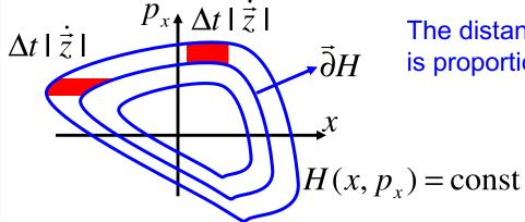
The distance d of lines with equal energy is proportional to  $1/|\vec{\partial}H| \propto |\vec{z}|^{-1}$
