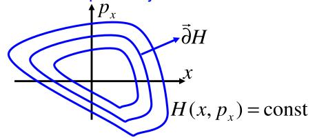
$$\frac{d}{ds}\vec{z} = \underline{J} \,\vec{\partial} H \quad \Rightarrow \quad \frac{d}{ds}\vec{z} \perp \vec{\partial} H$$
