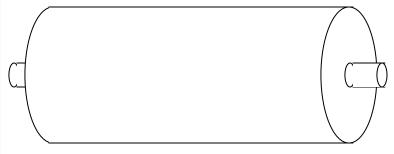
$$\omega_{nm}^{(E/B)} = c\sqrt{k_{nm}^{(E/B)2} + \left(\frac{l\pi}{L}\right)^2}$$
