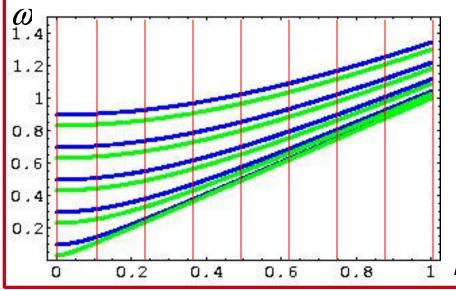
For each mode TE<sub>nm</sub> or TM<sub>nm</sub> there is a discrete set of frequencies that can be excited.
