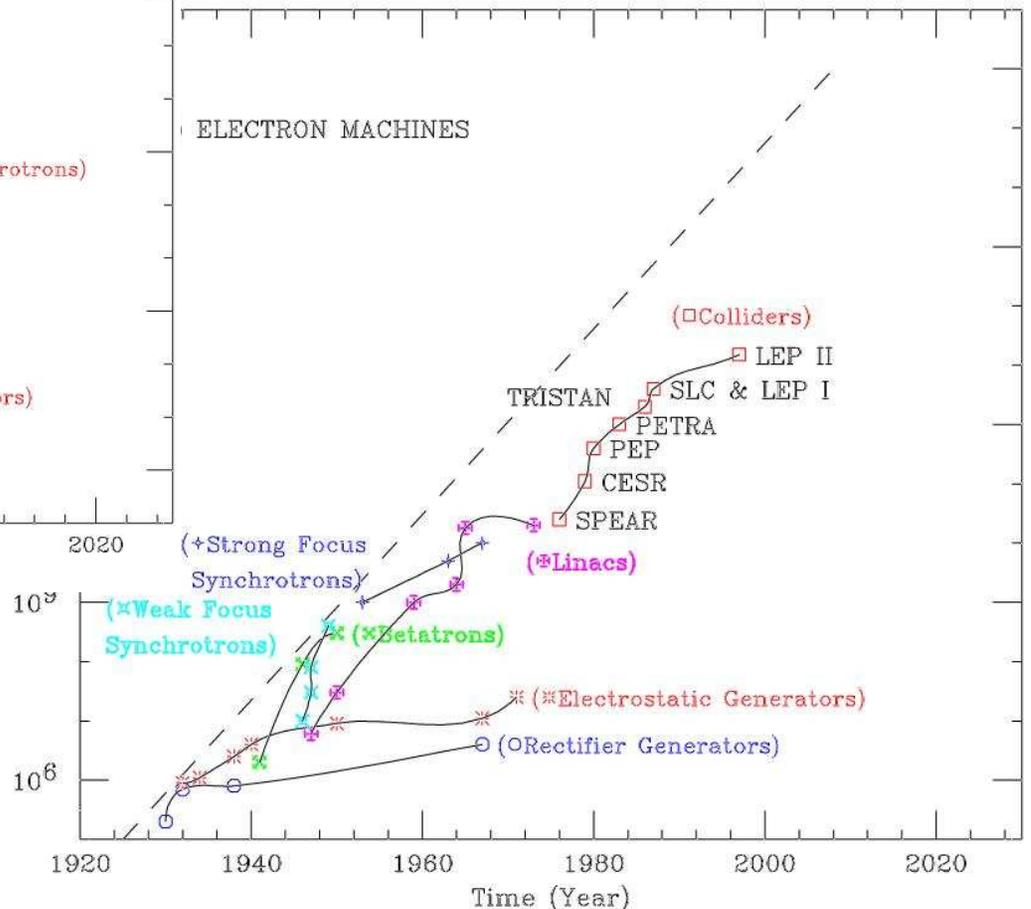
Energy that would be needed in a fixed target experiment versus the year of achievement
