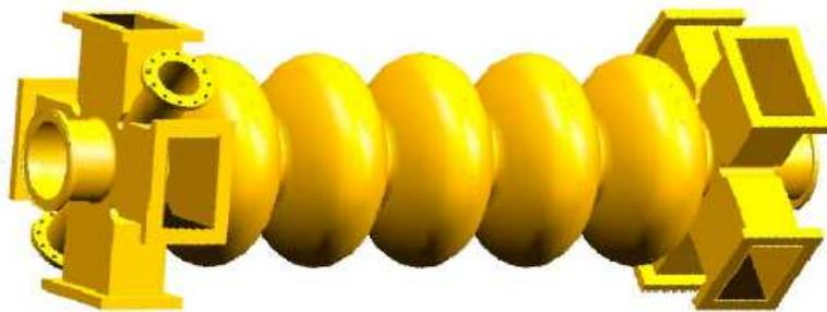
5-cell waveguide damped cavity
