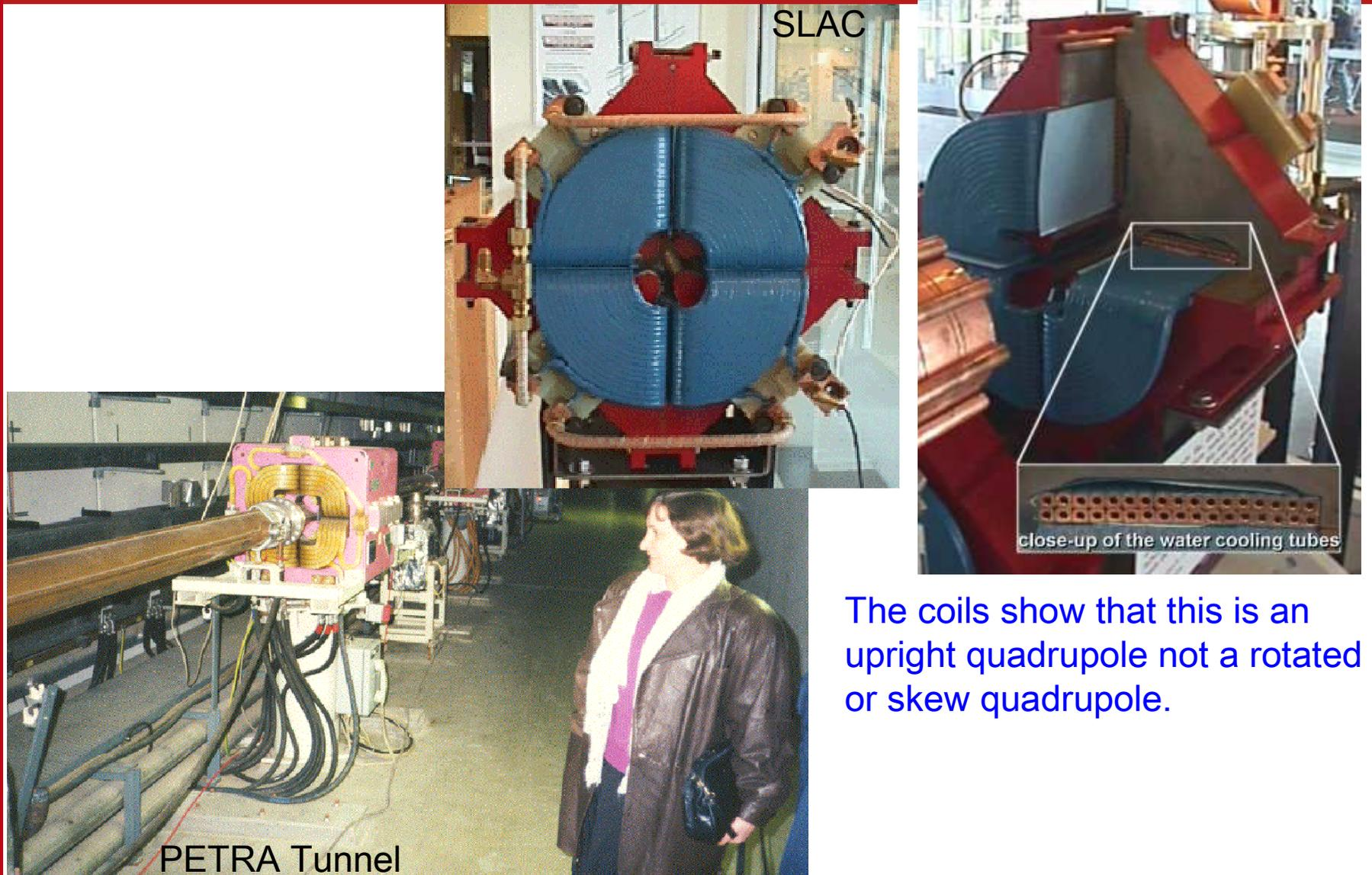
The coils show that this is an upright quadrupole not a rotated or skew quadrupole.
