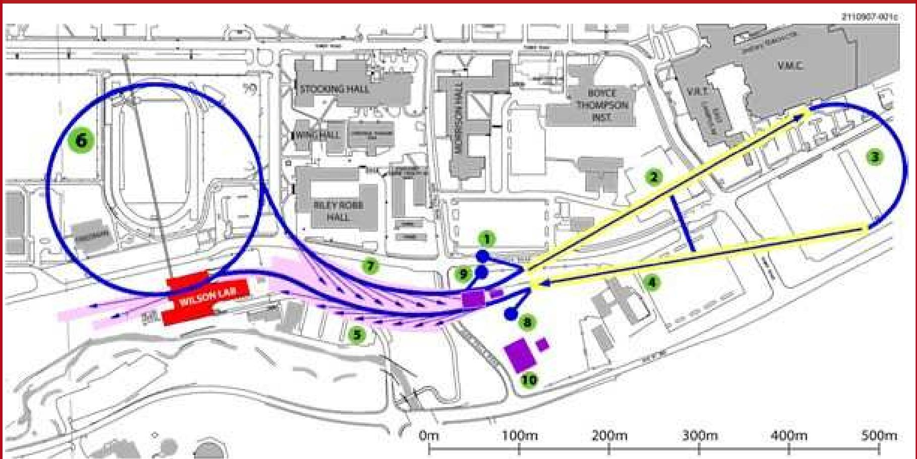
**Key:** 1) injector, 2) north linac, 3)turn-around arc, 4) south linac, 5) south x-ray beamlines, 6) CESR turn-around, 7) north x-ray beamlines, 8) 1<sup>st</sup> beam dump, 9) 2<sup>nd</sup> beam dump and 10)distributed cryoplant. Tunnel cross-section of 12' ID shown on lower right.
