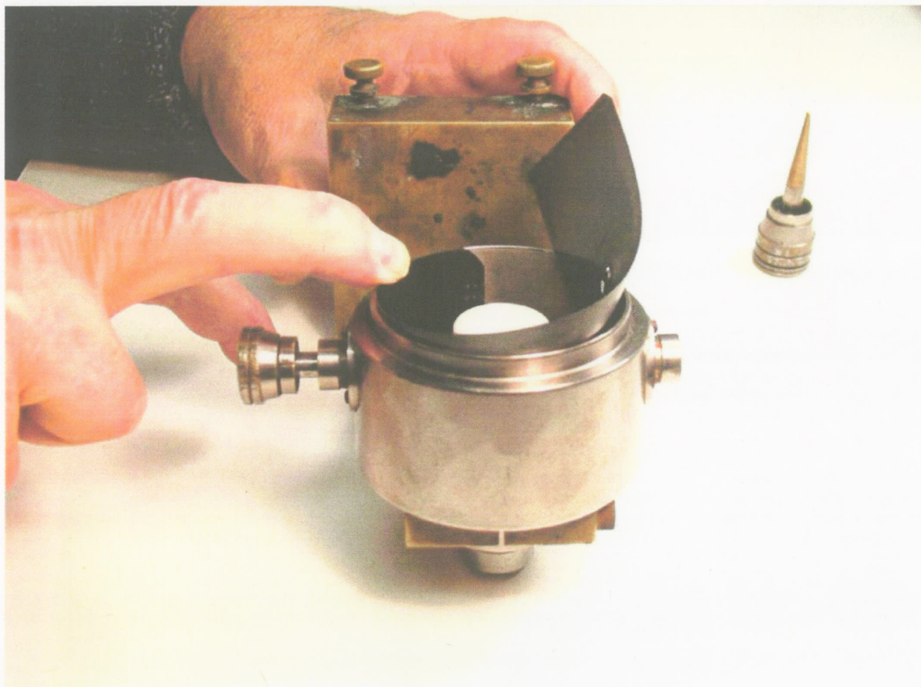
Inserting the film. Use collimator to help hold it in place.
