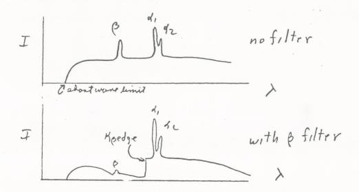
The  $K_{\beta}$  line of the target is effectively removed, but in the vicinity of the  $\alpha$  lines there is a sharp discontinuity due to the K edge of the filter. Now, any powder line is really a wavelength analysis of the tube spectrum and hence will show the edge. For low angle reflections the edge will be close to the  $\alpha$  doublet, whereas for higher angle lines it will be progressively further away. This is shown schematically below:
