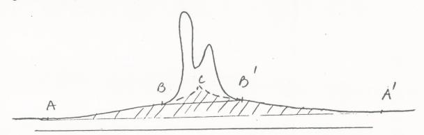
It has been shown\* that most of the tail region is due to thermally diffuse scattered x-rays (TDS). The approximate shape of this scattering is ABCB'A' in the figure. The correction due to thermal scattering taking the background at AA' is the hatched area in the figure and depending on the order of the reflection and the elastic softness of the crystal can range from a few percent to upwards of 20 to 30%. In the present case the corrections would be relatively small.
