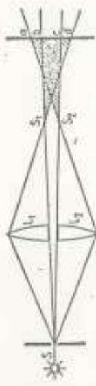
FIG. 13P. Diagram of Billot's split beam for producing interference fringes.
