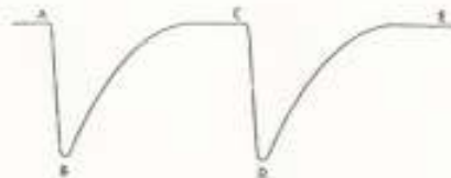
Fig. 4. The oscilloscope trace for two passages through zero field.
