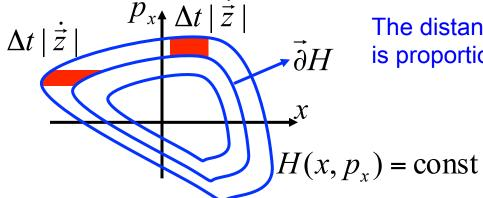
The distance d of lines with equal energy is proportional to  $d \propto 1/\|\vec{\partial} H\| \propto \|\vec{z}\|^{-1}$
