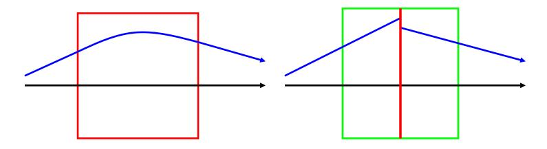
$$\vec{z}(s) = \underline{M}(s)\vec{z}_0 = \underline{D}(\frac{s}{2})\underline{D}^{-1}(\frac{s}{2})\underline{M}(s)\underline{D}^{-1}(\frac{s}{2})\underline{D}(\frac{s}{2})\vec{z}_0$$
