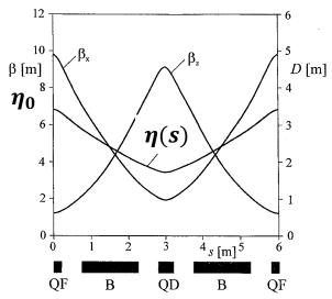
The dispersion that starts with 0 is called D(s), the dispersion that is periodic in a section is called  $\eta(s)$ .
