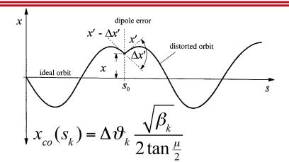
$$x_{co}(s) = \Delta \vartheta_k \frac{\sqrt{\beta \beta_k}}{2 \sin \frac{\mu}{2}} \cos(\left| \psi - \psi_k \right| - \frac{\mu}{2})$$
