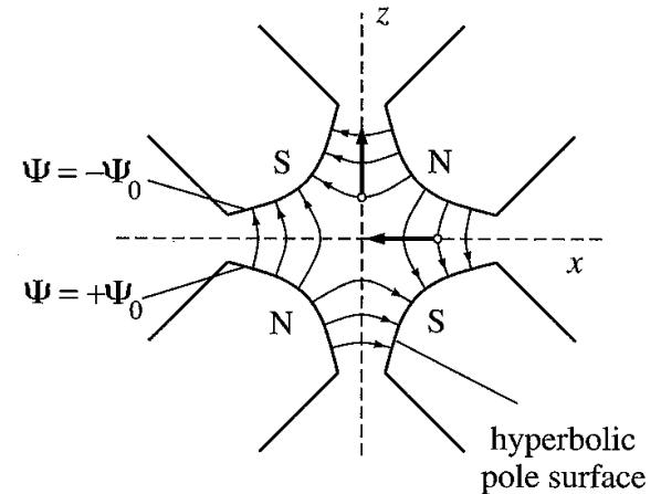
For positive  $k$ , focusing in x and defocusing in y.
