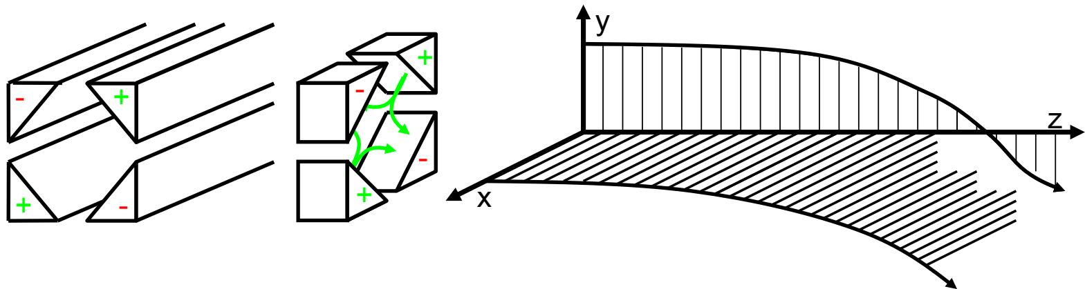
In a **quadrupole** particles are focused in one plane and defocused in the other plane. Other modes of **strong focusing** are not possible.
