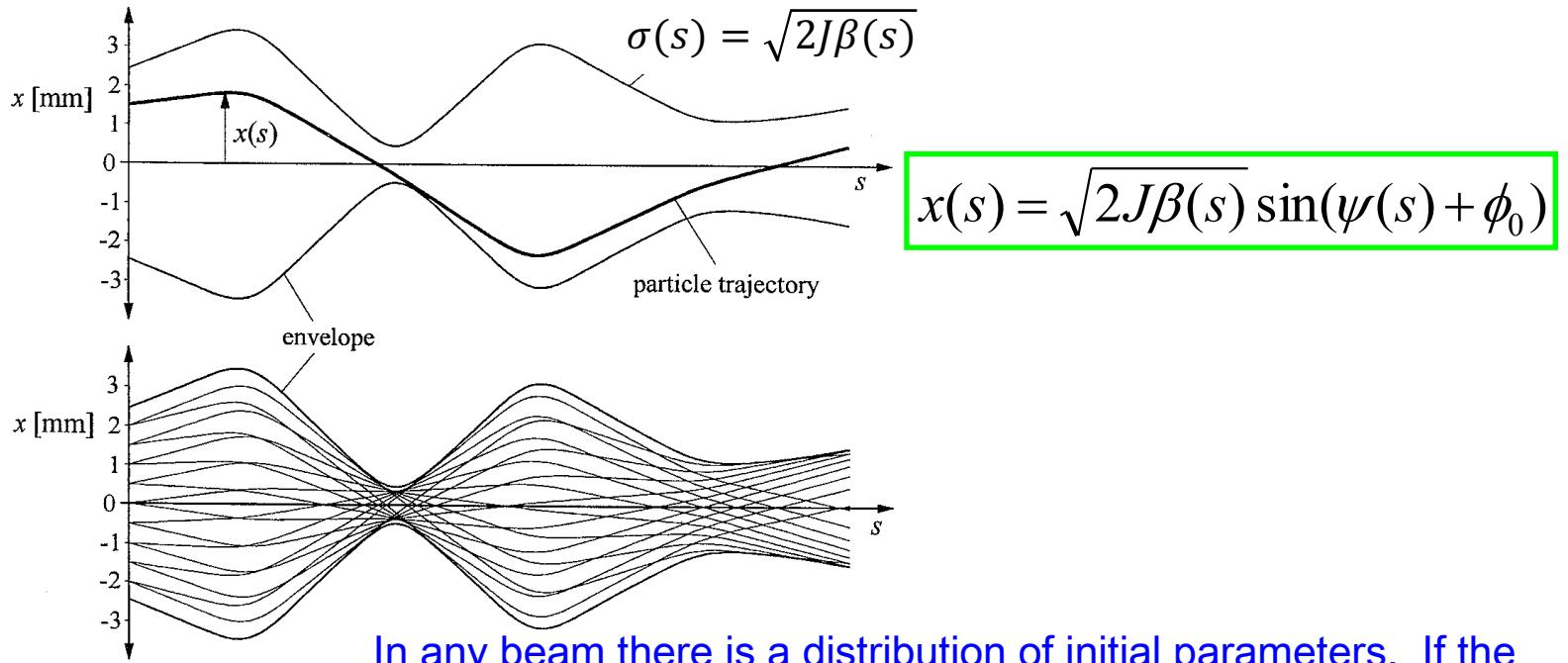
In any beam there is a distribution of initial parameters. If the particles with the largest  $J$  are distributed in  $\phi$  over all angles, then the envelope of the beam is described by  $\sigma = \sqrt{2J_{max}\beta(s)}$ . The initial conditions of  $\beta$  and  $\alpha$  are chosen so that this is approximately the case.
