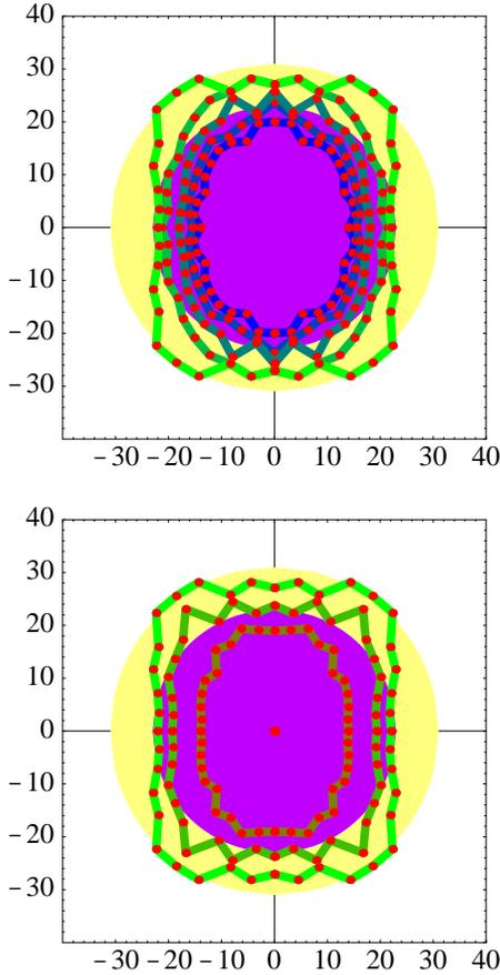
Figure 1: The boundaries of stable motion in  $x$  and  $y$  shown in units of beam sigmas for the  $72^\circ$  lumi upgrade optics with rf frequency shift for energy deviations top: from 0% (green) to 1% (blue) in intervals of 0.25%, bottom: from 0% (green) to -0.5% (red). An energy shift of -0.75/tune is not rematched.
