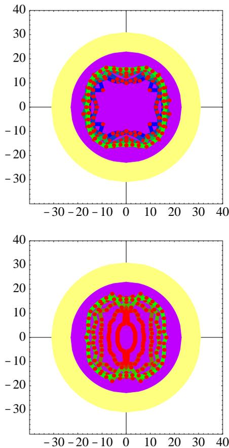
Figure 3: The boundaries of stable motion in  $x$  and  $y$  shown in units of beam sigmas for the  $72^\circ$  lumi upgrade optics with rf frequency shift and chromatic correction for energy deviations top: from 0% (green) to 1% (blue) in intervals of 0.25%, bottom: from 0% (green) to -1% (red).
