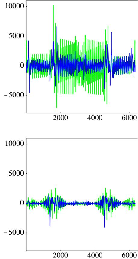
Figure 2: The energy dependence of the beta function  $\partial_\delta\beta_x$  and  $\partial_\delta\beta_y$  before chromatic correction (top) and after chromatic correction (bottom). The beta beat is matched to zero at the IPs and at the center of the arcs.
