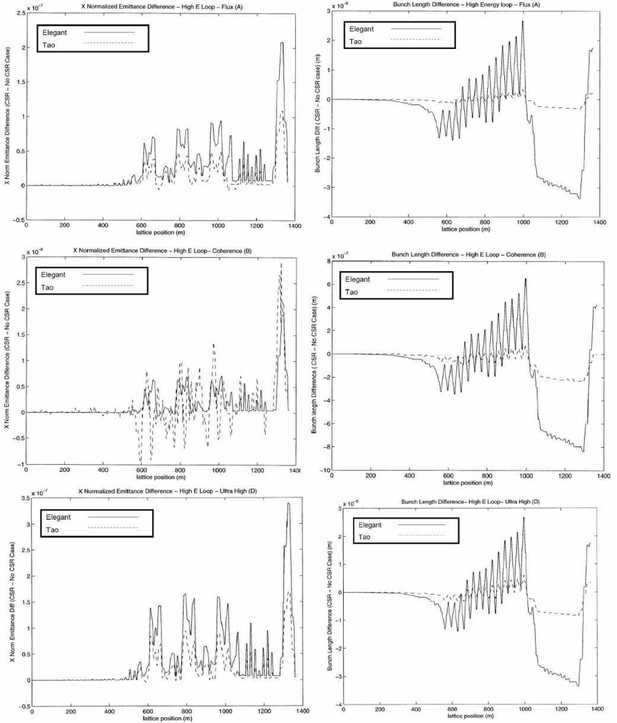
FIG. 7: Plots of Bunch length and X Normalized Emittance vs lattice position in the High Energy Loop for each of the three operating modes (A)-top, (B)-middle, (D)-Bottom.
