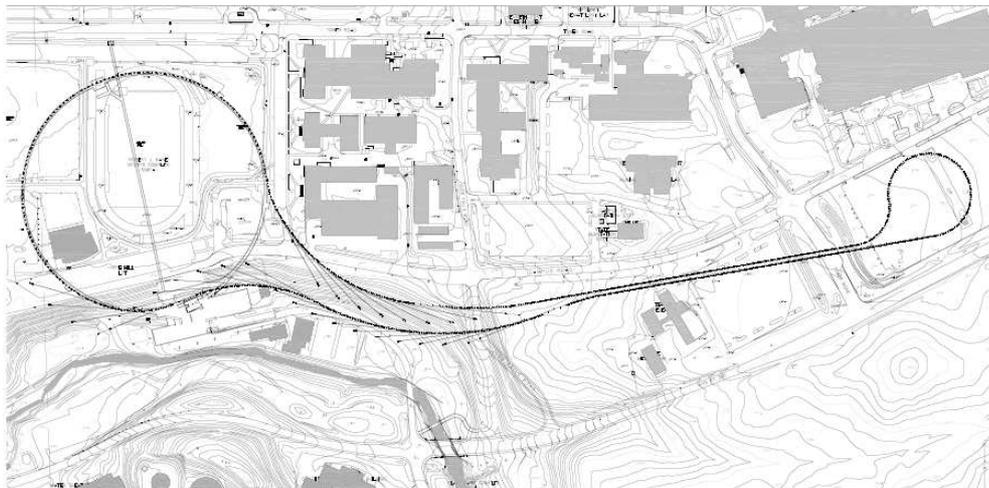
FIG. 2: ERL lattice modeled in TAO and ELEGANT: The turnaround section to the right of the figure and the High Energy loop to the left of the figure. The Short bunch section is located along the beam lines of the Northern Arc
