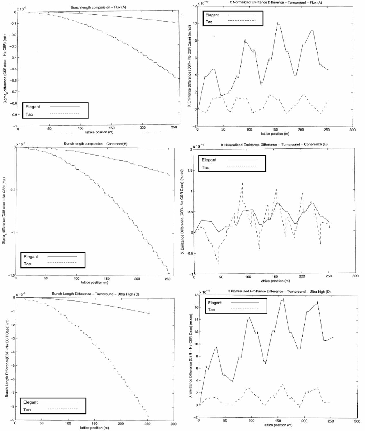
FIG. 5: Plots of bunch length and emittance vs lattice position in the Turnaround Section for each of the three operating modes (A)-top, (B)-middle, (D)-Bottom.
