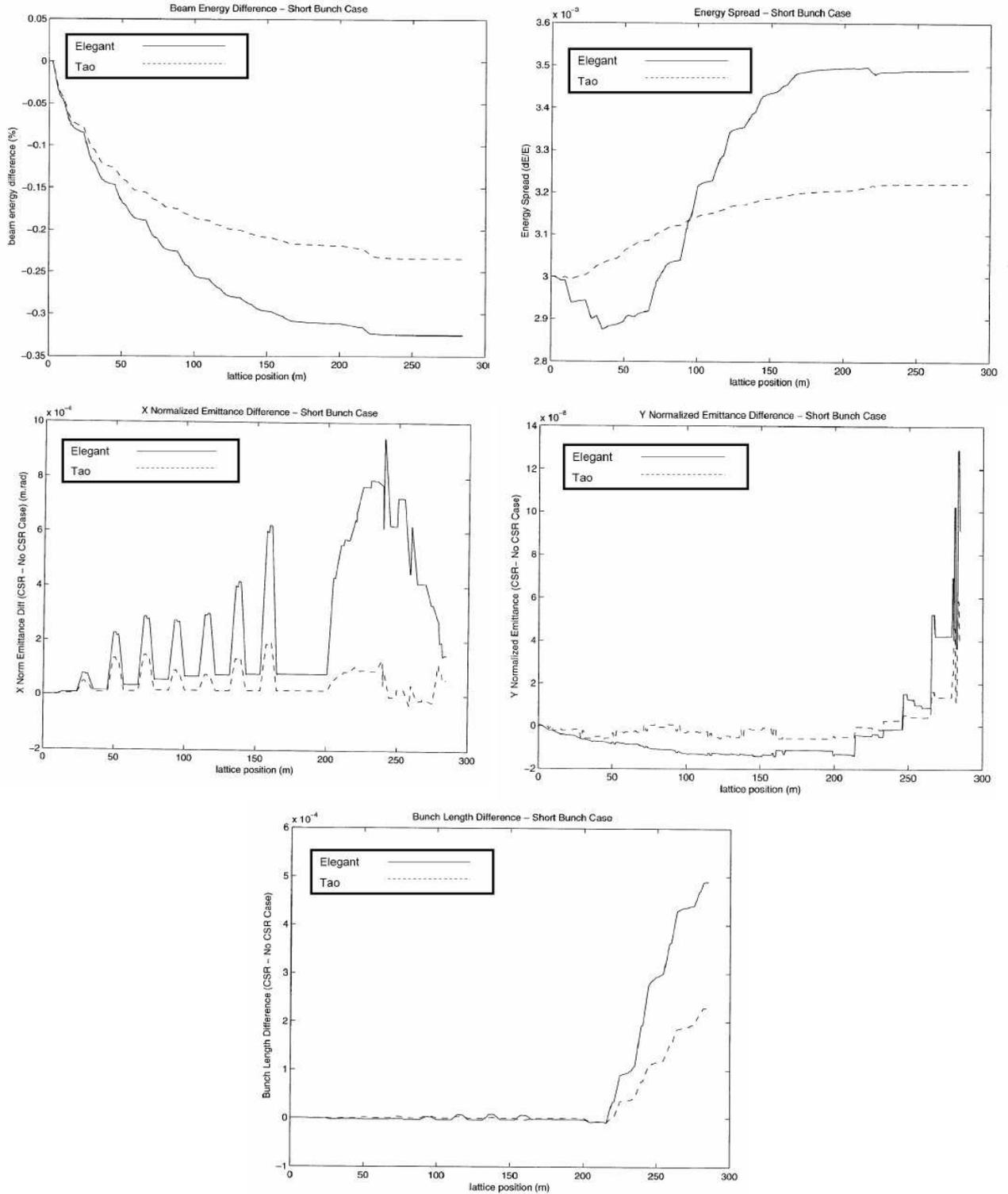
FIG. 8: Plots of compared beam parameters vs lattice position in the North Arc undulator section of the ERL under the "Short Bunch" operating modes.
