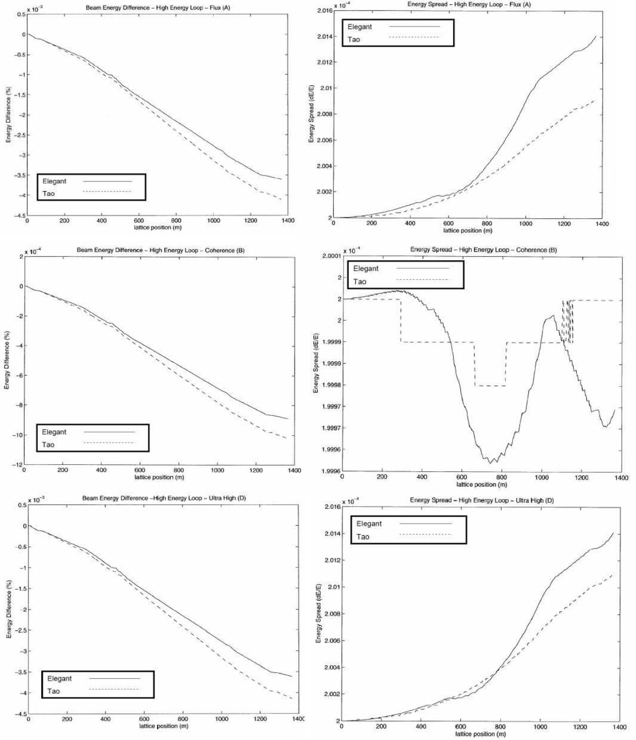
FIG. 6: Plots of Energy Spread and Energy Difference vs lattice position in the High Energy Loop for each of the three operating modes (A)-top, (B)-middle, (D)-Bottom.
