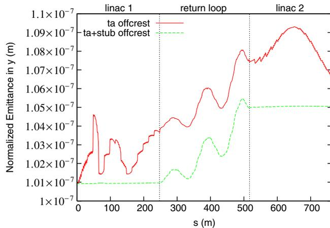
FIG. 8. (Color) Emittance growth with off-crest operation with and without symmetrizing stub.
