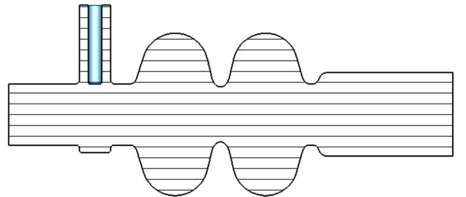
FIG. 7. (Color) Accelerating cavity with 1 cm symmetrizing stub.
