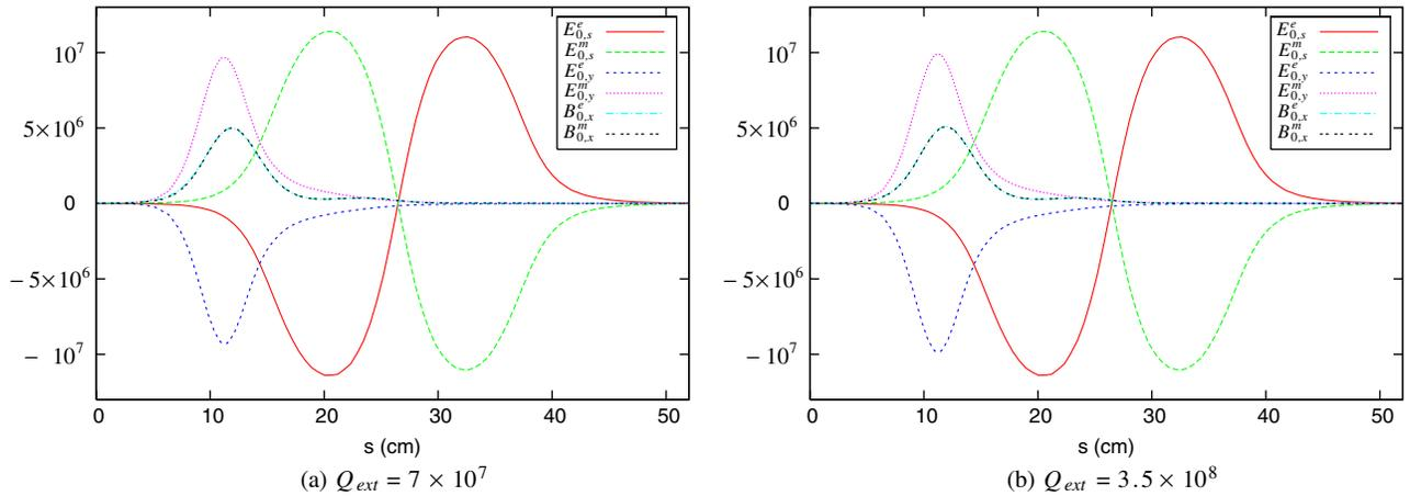
FIG. 2. (Color) Field profiles of MWS standing waves for  $Q_{\text{ext}}$  values of  $7 \times 10^7$  and  $3.5 \times 10^8$ . Units are MV/m and T for the electric and magnetic fields, respectively.  $E_{0,y}^e$  and  $E_{0,y}^m$  are scaled by  $10^3$  and  $B_{0,x}^e$  and  $B_{0,x}^m$  are scaled by  $10^9$ . The standing wave approximation is justified with  $\mathbf{E}_0^m \approx -\mathbf{E}_0^e$  and  $\mathbf{B}_0^m \approx \mathbf{B}_0^e$ .
