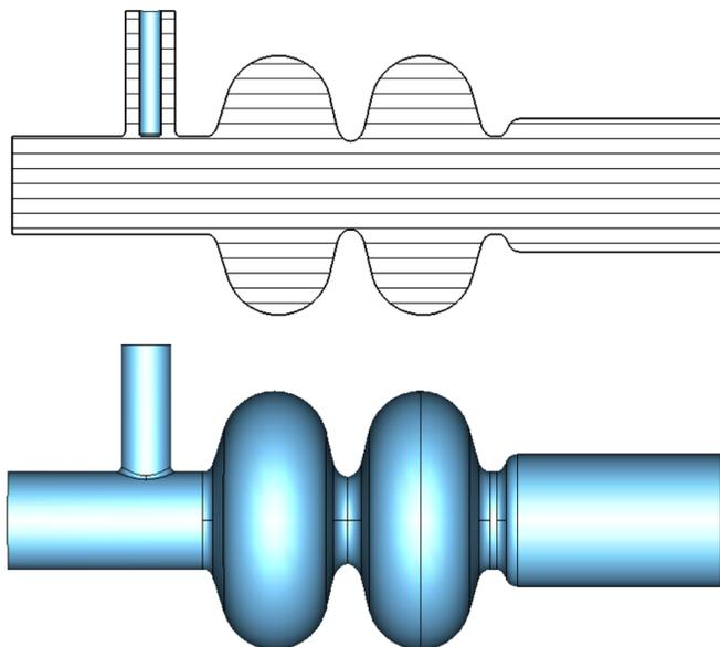
FIG. 1. (Color) Two cell model of the seven cell TESLA-type Cornell ERL superconducting rf cavity.
