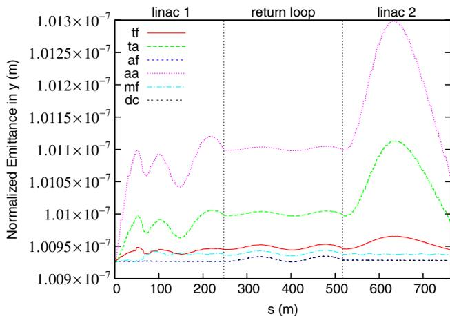
FIG. 5. (Color) Normalized emittance in the  $y$  direction for the six coupler configurations for  $Q_{\text{ext}} = 7 \times 10^7$ .
