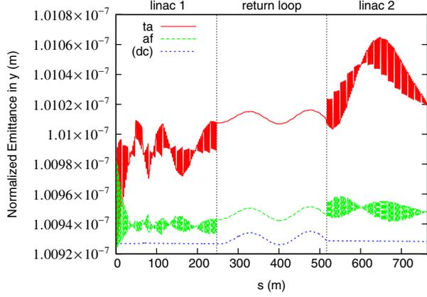
(c) Small emittance growth configurations,  $Q_{ext} = 3.5 \times 10^8$
