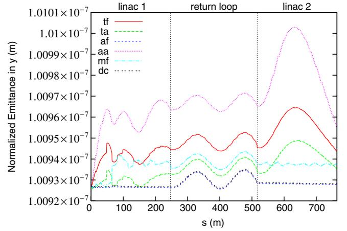
FIG. 6. (Color) Normalized emittance in the  $y$  direction for the six coupler configurations for  $Q_{\text{ext}} = 3.5 \times 10^8$ .
