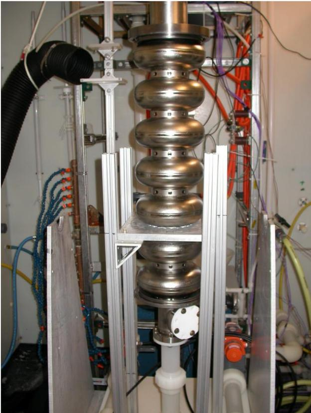
Figure 3: First Cavity Prepared for Vertical Test
