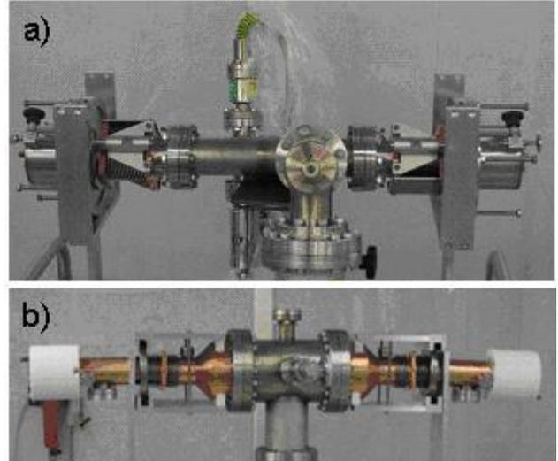
Figure 7: a) Cold and b) Warm Coupler Bake Assemblies at Daresbury
