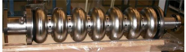
Figure 1: 7-cell cavity after final electron-beam welding.
