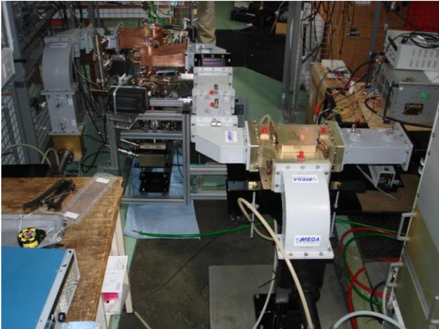
Figure 9: High Power Coupler Test Stand
