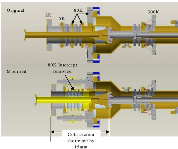
Figure 6: Original and Modified Cornell ERL Injector Coupler
