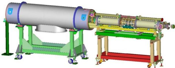
Figure 10: Cavity String Assembly into Outer Cryomodule
